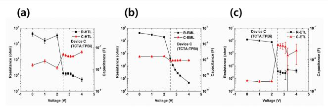
Fig. 9 Resistance-voltage-capacitance simulation results for each organic layer. (a) HTL, (b) EML, and (c) ETL. Reproduced with permission from ref. 37 Copyright 2023, Elsevier Ltd
