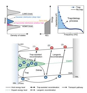
Fig. 10 Trap dynamics and recombination mechanisms: energy distribution of density of states (DOS) in the host and dopant with Fermi-Dirac distribution, the contribution of trap dynamics on the capacitance-frequency spectrum, and the schematic diagram illustrating the trap-assisted and Langevin recombination ( $\gamma_L$ ) processes. Reproduced with permission from ref. 57 Copyright 2023, Wiley-VCH.
