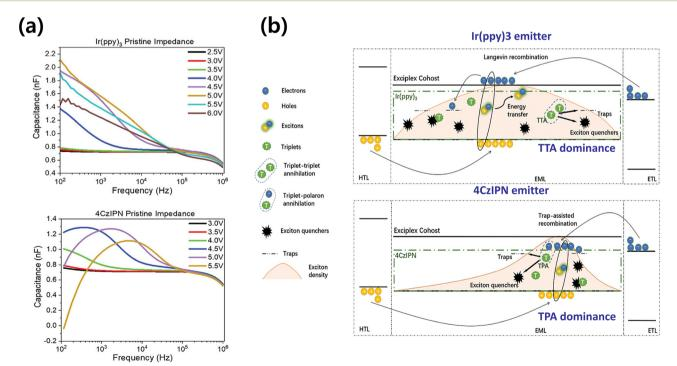
Fig. 17 (a) Capacitance-frequency plot of the Ir(ppy)<sub>3</sub>- and 4CzIPN-based devices. (b) TTA and TPA degradation and quenching mechanisms in a phosphorescent emitter (Ir(ppy)<sub>3</sub>) and thermally activated delayed fluorescent emitter (4CzIPN), respectively. Reproduced with permission from ref. 58 Copyright 2024, Wiley-VCH.
