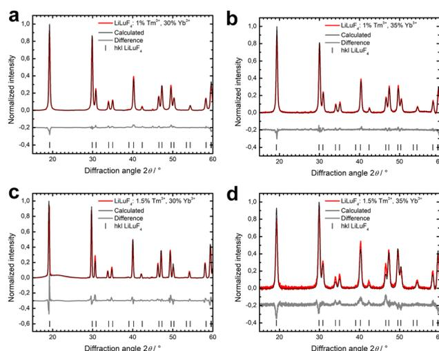
Fig. 3 Rietveld refinement of the PXRD patterns ( $Cu K\alpha$  radiation) of the  $LiLuF_4:Tm^{3+}, Yb^{3+}$  NCs with different activator ratios of  $Tm$  and  $Yb$ .  $LiLuF_4$  (#PDF 00-027-1251).<sup>54</sup> (a) 1%  $Tm^{3+}$ , 30%  $Yb^{3+}$ , (b) 1%  $Tm^{3+}$ , 35%  $Yb^{3+}$ , (c) 1.5%  $Tm^{3+}$ , 30%  $Yb^{3+}$ , and (d) 1.5%  $Tm^{3+}$ , 35%  $Yb^{3+}$ .
