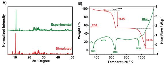
Fig. 3 (A) Room temperature PXRD pattern of 1 powder as well as the simulated pattern from SCXRD. (B) TGA-DSC thermograms of 1 in a nitrogen atmosphere.
