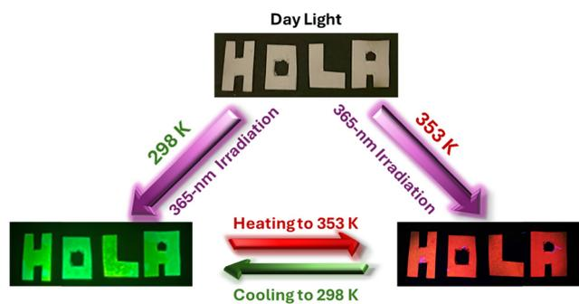
**Scheme 1** Illustration of a dual-key encryption–decryption thermophotochromic phenomenon using heat and light to read codes (two colours) in a single compound, **1**, adsorbed on a white filter paper.
