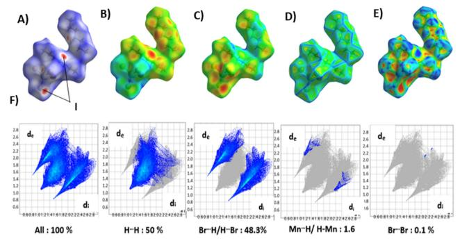
Fig. 2 3D Hirshfeld surfaces mapped over (A):  $d_{norm}$  (close contacts are presented by red spots), (B)  $d_{ir}$  (C)  $d_{er}$  (D) curvedness, (E) shape index representations (F) 2D fingerprints resolved into all,  $H \cdots H$ ,  $Br \cdots H/H \cdots Br$ ,  $Mn \cdots H/H \cdots Mn$  and  $Br \cdots Br$  contacts, showing the contribution to the total Hirshfeld surface area
