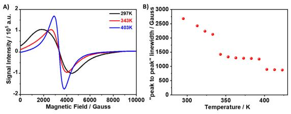
(A) X-band EPR spectra of 1 recorded at different temperatures. (B) Thermal evolution of the "peak-to-peak" linewidth.
