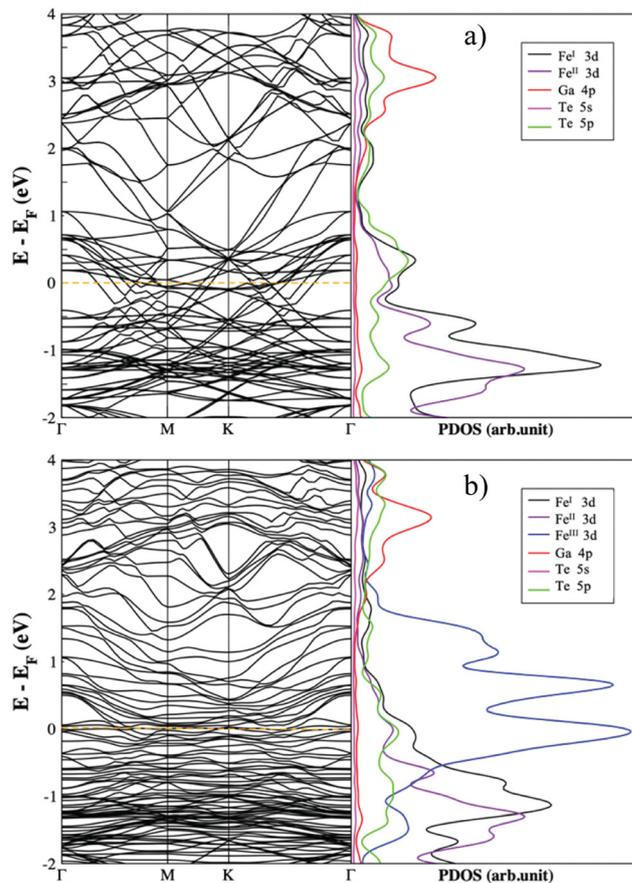
Fig. 4 The band structure and projected density of states (a) of ideal  $\text{Fe}_3\text{GaTe}_2$  (FGaT) and (b)  $\text{Fe}_3\text{GaTe}_2$  (FGaT) with 12.5% interstitial iron occupancy. The orange dashed line on the left-hand side of each plot represents the Fermi level at 0 eV.
