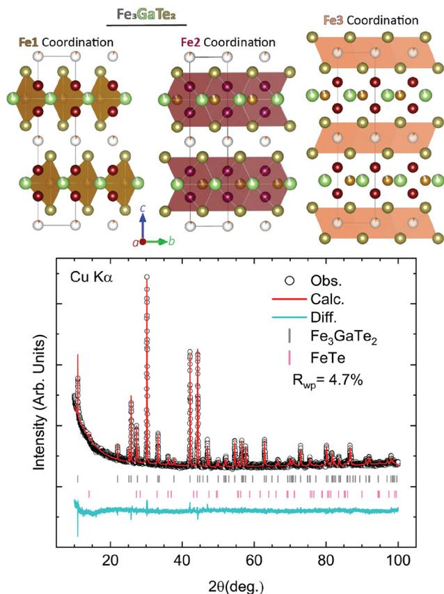
**Fig. 1** The structural model of  $\text{Fe}_3\text{GaTe}_2$  and powder diffraction data with X-rays. The three representations of the crystal show the iron in 3 different coordination geometries: Fe1, Fe2, and Fe3. Both Fe1 and Fe3 are not fully occupied, and Fe3 is considered interstitial. Rietveld refinement of the structure fitted to powder XRD using Cu K $\alpha$  radiation ( $\lambda_1 = 1.540562 \text{ \AA}$ / $\lambda_2 = 1.544398 \text{ \AA}$ ).
