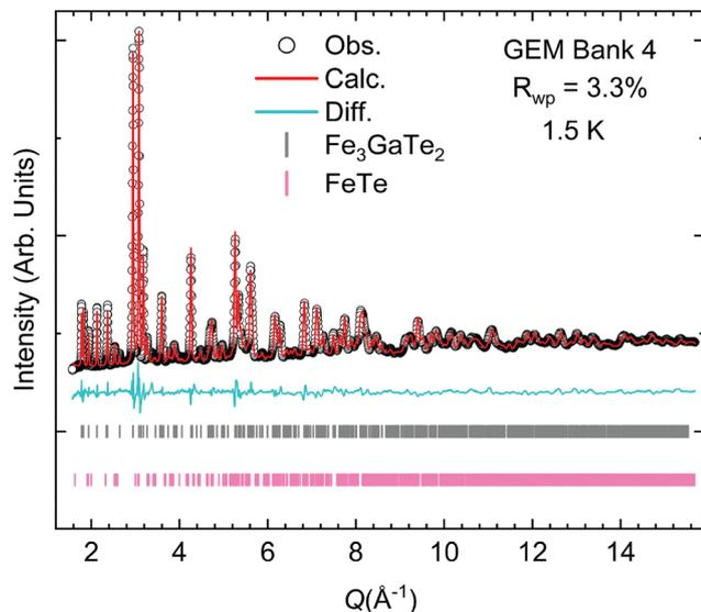
Fig. 2 Neutron powder diffraction (NPD) pattern of  $\text{Fe}_3\text{GaTe}_2$  at 1.5 K. The Rietveld refinement was performed using the structural model obtained from X-ray diffraction studies, and the magnetic space group was used to fit the magnetic intensity of the low- $Q$  reflections. The NPD was collected at the GEM beamline, which is a time-of-flight diffractometer. The impurity phase was found to be  $\text{Fe}_{1+x}\text{Te}$ , which was nearly 10 wt%.
