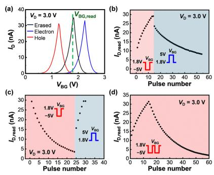
Fig. 3 (a) I<sub>D</sub>-V<sub>BG</sub> curves at the erased (black line), electron-trapped (blue line), and hole-trapped (red line) states. (b) LTP and LTD operations as a function of presynaptic pulse numbers, with the electron-trapped state defined as the initial state. (c) LTD and LTP as a function of presynaptic pulse numbers, following an erasing operation. I.e., no carriers were trapped in the Au FG. (c) Transition from LTP to LTD induced by continuous presynaptic pulses.
