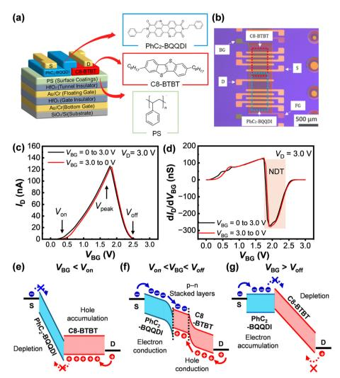
Fig. 1 (a) Device structure and (b) optical microscope image of the FG-OAAT, utilizing PhC2-BQQDI and C8-BTBT films as transistor channels, with an Au film serving as the floating gate. (c)  $I_D - V_{BG}$  and (d) differential transconductance curve of the FG-OAAT measured at  $V_D = 3.0$  V. (e) Illustrations of carrier transport in the FG-OAAT across  $V_{BG}$  ranges: (a)  $V_{BG} < V_{Onr}$ , (b)  $V_{on} < V_{BG} < V_{off}$ , and (c)  $V_{off} < V_{BG}$ .
