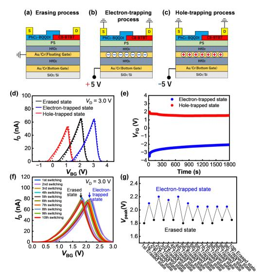
Fig. 2 (a) Erasing, (b) electron-trapping, and (c) hole-trapping processes of the FG-OAATs. (d)  $I_D - V_{BG}$  curves for the erased (black line), electron-trapped (blue line), and hole-trapped (red line) states, with solid and dotted lines representing forward and reverse  $V_{BG}$  sweeps, respectively. (e) Retention property of the FG-OAAT. (f) Switching behavior of the FG-OAAT. (g) Variation in  $V_{\rm peak}$  values in electron-trapped and erased states as a function of switching cycles.
