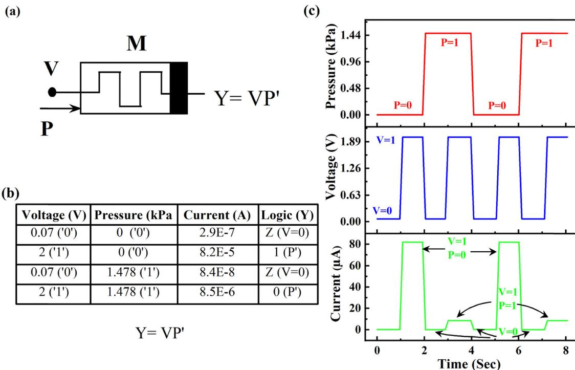
Fig. 8 (a) Schematic of memristor with applied pressure (b) truth table of the device derived from the  $I-V$  characteristics (c) output current levels as a result of different combinations of applied electrical and pressure logic inputs, read at 2 V with threshold current set to 10  $\mu\text{A}$ .
