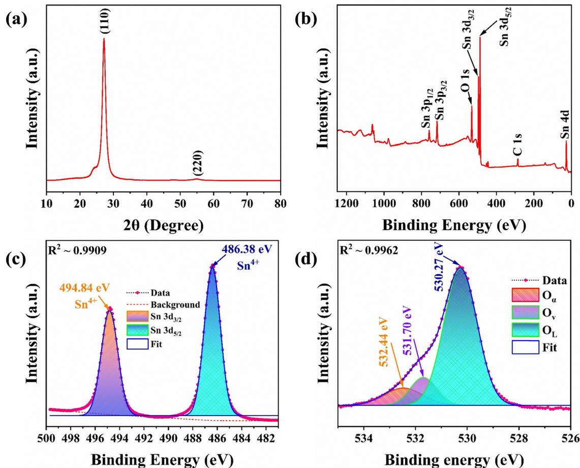
Fig. 1 (a) XRD spectra of tin oxide ( $\text{SnO}_{2-x}$ ) film, synthesized by the hydrothermal method. (b) X-ray photoelectron spectroscopy (XPS) survey spectra of  $\text{SnO}_{2-x}$  spin-coated film, (c) and (d) deconvoluted XPS spectra of Sn 3d and O 1s peaks in  $\text{SnO}_{2-x}$  film, respectively.
