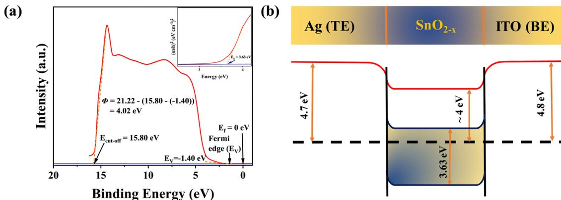
Fig. 3 (a) Work function and band gap estimation of  $\text{SnO}_{2-x}$  film using UPS result and Taucs plot (inset) respectively, (b) band diagram of Ag/ $\text{SnO}_{2-x}$ /ITO memristive device under equilibrium.
