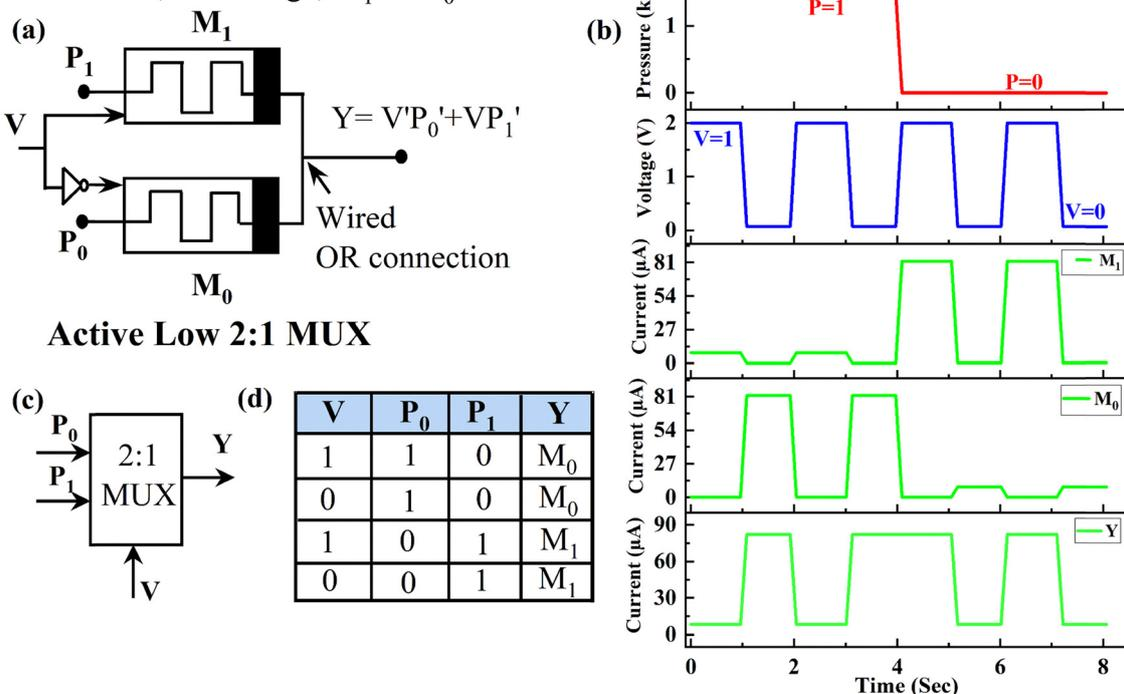
Fig. 9 (a) Proposed active-low 2:1 MUX logic circuit with the fabricated memristor. (b) The timing diagram of current levels with the pressure of the proposed MUX logic circuit derived from the  $I-V$  characteristics (c) Schematic of the proposed active low 2:1 MUX logic (d) truth table of the proposed MUX.
