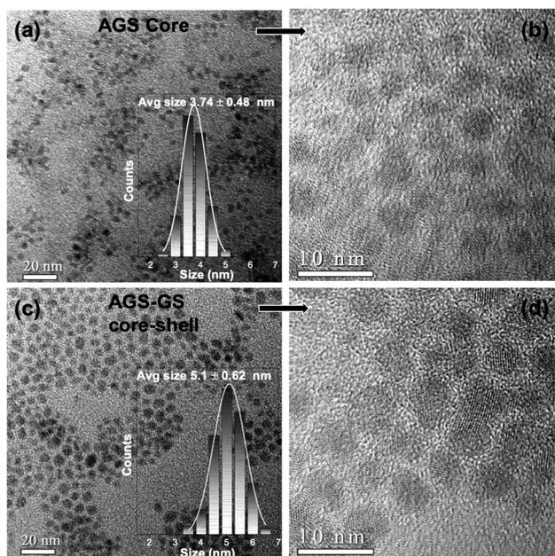
**Fig. 3** TEM (a), (c) and HRTEM (b), (d) images of core AGS (a), (b) and core-shell AGS-GS QDs (c), (d), respectively. Insets of (a) and (b) show the corresponding size distributions and calculated average size.
