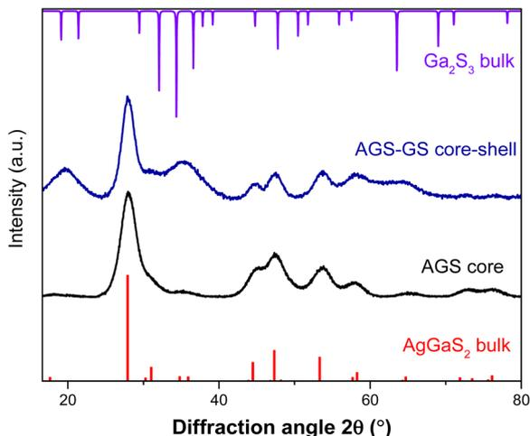
Fig. 4 XRD patterns of the AGS core and AGS-GS core-shell QDs in comparison with bulk  $\text{AgGaS}_2$  in the tetragonal phase (ICSD 01-073-1233) and monoclinic  $\text{Ga}_2\text{S}_3$  (ICSD 00-050-0811) diffraction patterns from ICSD database.
