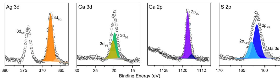
Fig. 5 High-resolution XPS spectra of Ag 3d, Ga 3d, Ga  $2p_{3/2}$ , and S 2p regions for (a) AGS core and (b) AGS-GS core-shell QDs. N.B.: the small peak visible at lower energies is related to the sample charging due to the presence of insulating organic ligands.
