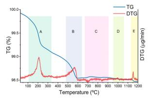
Fig. 4 Thermogravimetric and corresponding derivative curves for the LiYGeO<sub>4</sub> synthesis, starting from the precursor's powders in the used stoichiometry.
