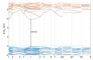
Fig. 2 Calculated band structure of LiYGeO<sub>4</sub> using the HSE06 hybrid functional. The indicated energy is the calculated bandgap value, the blue/red lines indicate the occupied/unoccupied electronic states, and the horizontal dashed line lies at the Fermi energy.
