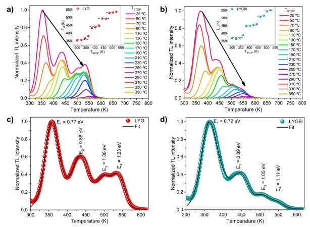
Fig. 8 Thermoluminescence study of the two produced samples (LYG and LYGBi) by the  $T_{M}$ - $T_{STOP}$  method (panels a and b) and by glow curve computational fitting (panels c and d). The insets in the upper panels show the evolution of the temperature position of the first,  $T_{Mr}$ , as a function of the pre-heating temperature,  $T_{\text{STOP}}$ , used to gradually depopulate the traps.
