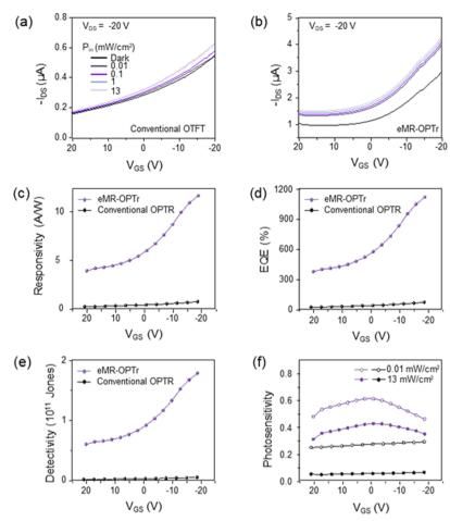
Fig. 5 (a) Transfer curve without eMR-gates; (b) Transfer curve with eMR-gates. (c-f) Performance of organic phototransistors with and without eMRqates: (c) R, (d) EQE, (e)  $D^*$ , and (f) S at light intensity of 0.01 mW cm<sup>-2</sup>. The device performance of the conventional OPTRs was extracted at  $V_{DS} = -80 \text{ V}$ , where the maximum response was observed
