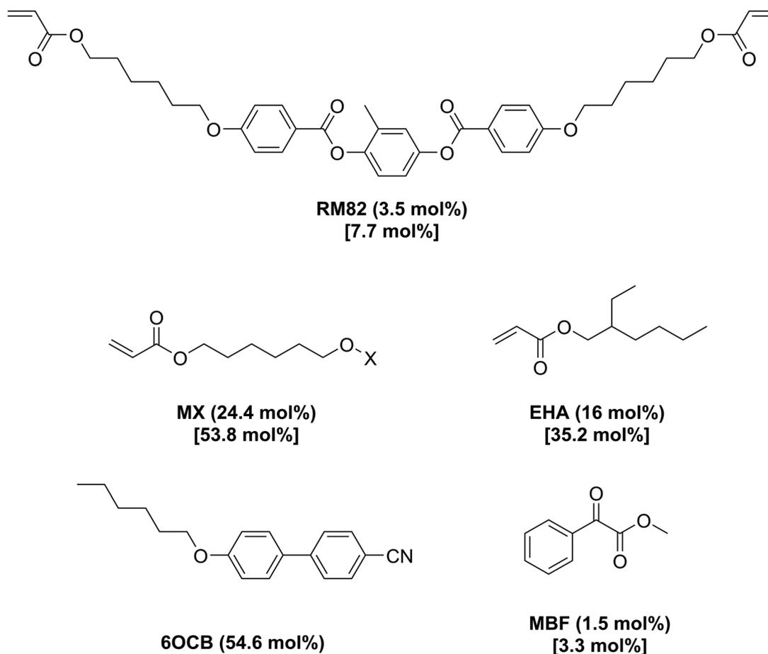
Fig. 3 Generalised composition of the LCE mixture when the monofunctional mesogenic monomer **MX** is varied. The quantities in square brackets denote the composition of the final LCE after the unreactive material has been removed. In the case of **MX**, the **X** displayed in the chemical structure, denotes the appropriate mesogenic unit from Fig. 2.
