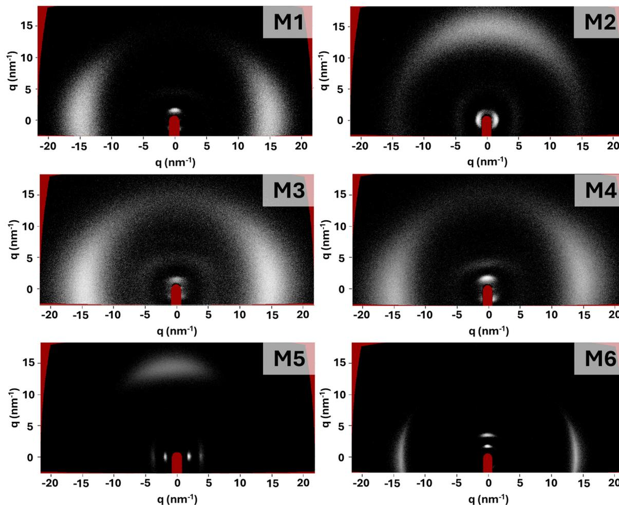
Fig. 4 Two-dimensional X-ray scattering data for each LCE sample. Planar samples were used, with the director approximately vertical (**M1**, **M3**, **M4** and **M6**) or horizontal (**M2** and **M5**). (001) Bragg peaks due to smectic layer spacing can be seen in each case close to the red beam stop. Only **M5** and **M6** show multiple small angle features (001) and (002) peaks.
