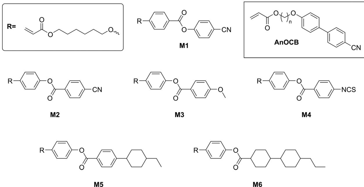
Fig. 2 The chemical structures of the monofunctional mesogenic monomer variations employed in the fabrication of LCEs within this work. The LCEs produced from the **AnOCB** monomers were reported previously<sup>4</sup> and differ by the number of repeat units in the spacer chain, as opposed to differences in the structure of the mesogenic unit as in **M1–M6**.
