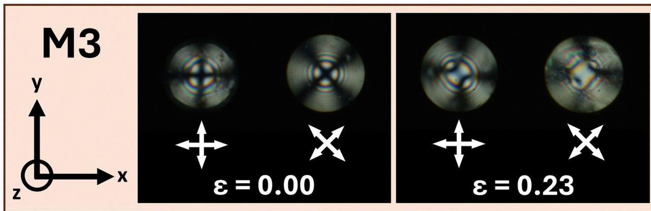
Fig. 6 Conoscopic figures for unstrained and strained samples of the LCE synthesised with **M3**. The strain applied ( $\epsilon$ ) and the orientation of the polarisers (denoted by the crossed white arrows) are reported for each image. Strain is applied in the  $x$  direction, as depicted by axes on the left-hand side of the figure.
