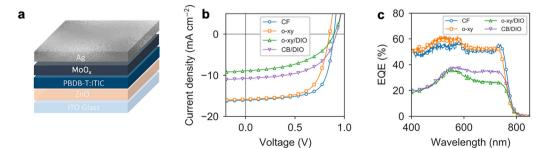
Fig. 4 (a) Inverted (n-i-p) organic solar cell device structure used in this work. (b) Champion J-V curves and (c) champion EQE spectra of the OPV devices prepared using four different co-solvent formulations.
