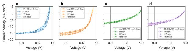
Fig. 6 J-V curves of the representative OPV devices processed from the different co-solvent formulations, as stored in the dark and in nitrogen for a period of 1322 days: (a) CF, (b) o-xy, (c) o-xy/DIO and (d) CB/DIO. Filled areas connect the first and last J-V curves
