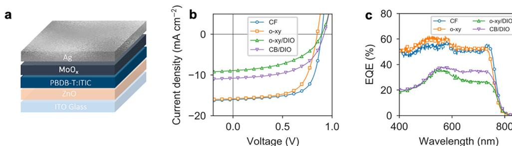
Fig. 4 (a) Inverted (n-i-p) organic solar cell device structure used in this work. (b) Champion *J*-*V* curves and (c) champion EQE spectra of the OPV devices prepared using four different co-solvent formulations.
