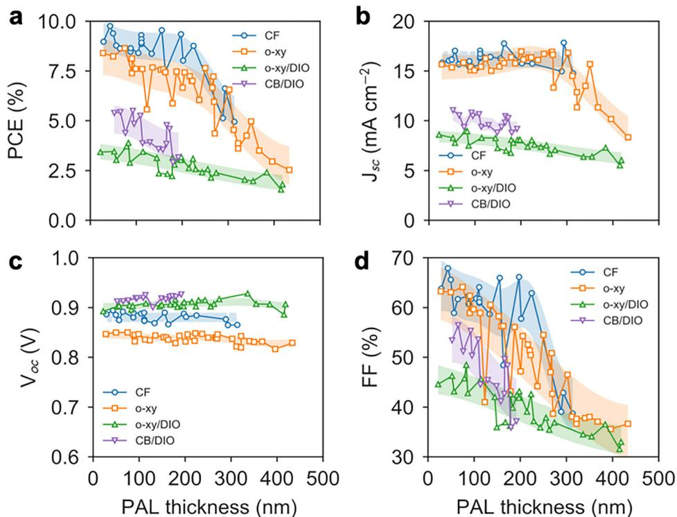
Fig. 5 Photovoltaic figures of merit as a function of the PAL thickness of the organic solar cells processed from the different co-solvent formulations used in this work. (a) PCE, (b)  $J_{sc}$ , (c)  $V_{oc}$  and (d) FF. In all cases, the shaded areas correspond to the native spread of support vector regression models that were fitted to the experimental data to serve as guide-to-the-eye.
