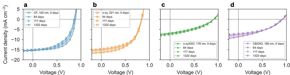
Fig. 6  $J$ - $V$  curves of the representative OPV devices processed from the different co-solvent formulations, as stored in the dark and in nitrogen for a period of 1322 days: (a) CF, (b) *o*-xy, (c) *o*-xy/DIO and (d) CB/DIO. Filled areas connect the first and last  $J$ - $V$  curves.
