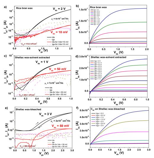
Fig. 14 (a) Transfer and (b) output characteristics of an OFET with  $C_{60}$  semiconductor and rice bran wax dielectric on plain aluminum gate electrode; (c) transfer and (d) output characteristics of an OFET with C<sub>60</sub> semiconductor and solvent extracted shellac wax dielectric on plain aluminum gate electrode; (e) transfer and (f) output characteristics of an OFET with  $C_{60}$  semiconductor and bleached shellac wax dielectric on plain aluminum gate electrode.
