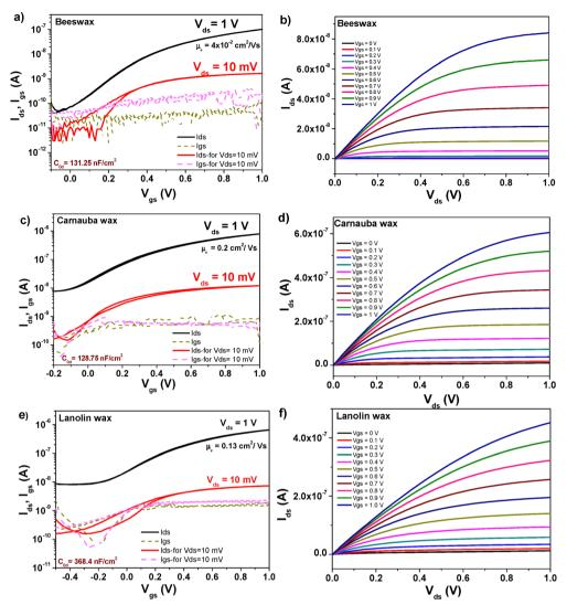
Fig. 13 (a) Transfer and (b) output characteristics of an OFET with C<sub>60</sub> semiconductor and beeswax dielectric on plain aluminum gate electrode; (c) transfer and (d) output characteristics of an OFET with C<sub>60</sub> semiconductor and carnauba wax dielectric on plain aluminum gate electrode; (e) transfer and (f) output characteristics of an OFET with  $C_{60}$  semiconductor and lanolin wax dielectric on plain aluminum gate electrode.
