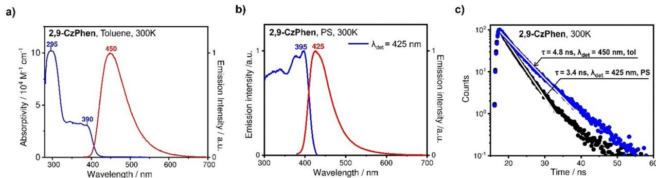
Fig. 7 (a) Absorption (blue) and emission (red) spectra of **2,9-CzPhen** in toluene ( $\approx 10^{-5}$  M) under ambient conditions. (b) Emission (red) and excitation (blue) spectra of **2,9-CzPhen** doped in PS film ( $\ll 1$  wt%). (c) Emission decay profiles of **2,9-CzPhen** in toluene ( $\approx 10^{-5}$  M) at ambient temperature (blue dots) and as doped in PS film (black dots) ( $\ll 1$  wt%).
