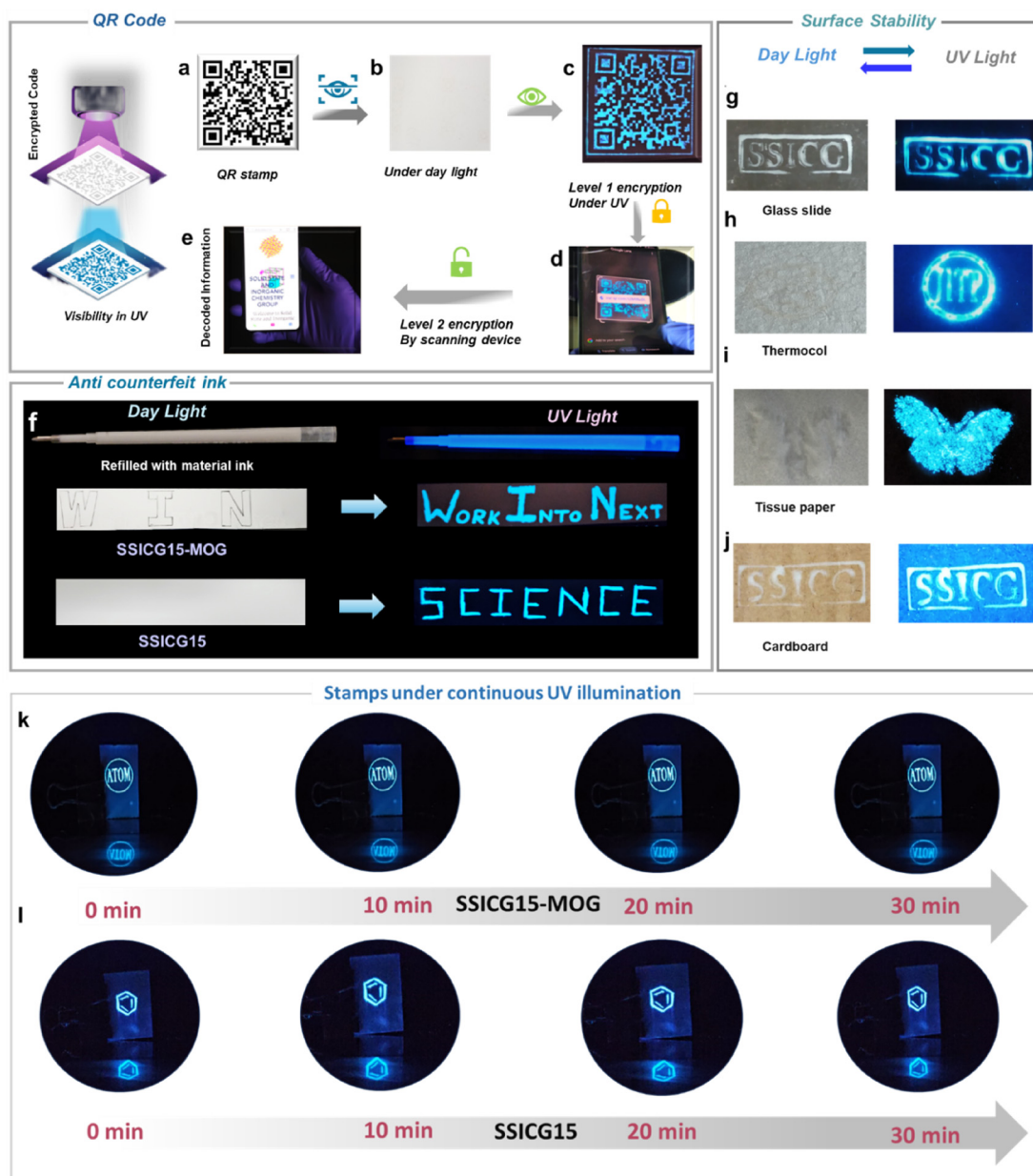
Fig. 4 (a) Image of the raw QR code; (b) stamped QR code in daylight; (c) visibility of the QR code in the presence of UV light; (d) image of the encrypted code while scanning with an electronic device; (e) image of decoded encrypted information; (f) image of the coded phrase (WORK INTO NEXT) with SSICG15-MOG and (SCIENCE) with SSICG15 using anticounterfeiting ink in the absence and presence of UV light; (g)–(j) anticounterfeiting stampings on different surfaces: (g) glass slide, (h) thermocol, (i) tissue paper, and (j) cardboard; (k) and (l) stability of SSICG15-MOG and SSICG15 in stamping under continuous UV irradiation.
