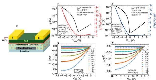
Fig. 4 FET characteristics with 5 nm  $\text{Al}_2\text{O}_3$ . (a) Device geometry with the addition of  $\text{Al}_2\text{O}_3$  layer. (b) and (c) Transfer and output characteristics of a DDP-DTT/PVDF-TrFE FET, respectively. (d) and (e) Transfer and output characteristics of a DDP-DTT/PVDF-HFP FET, respectively.
