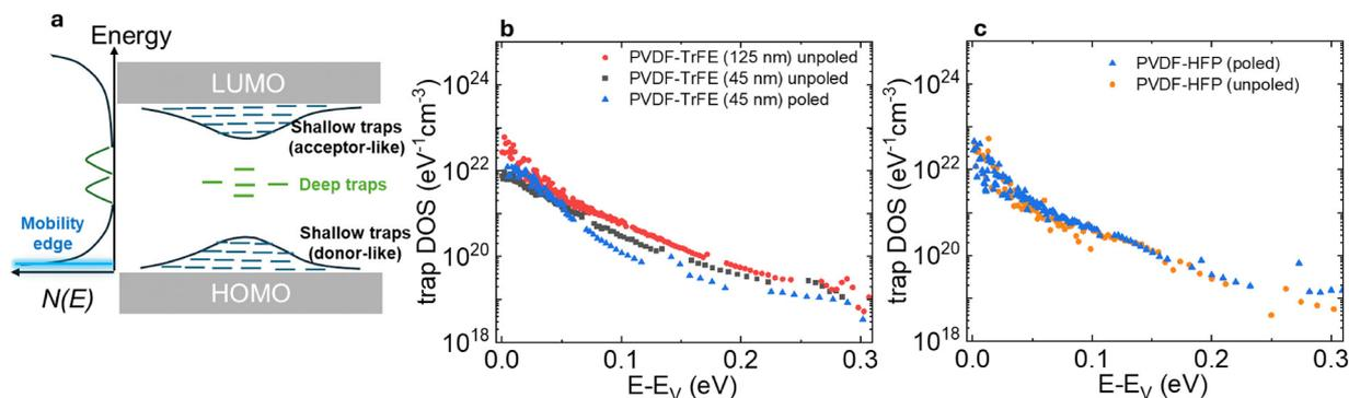
Fig. 3 Trap DOS in PVDF-TrFE and PVDF-HFP based DPP-DTT FETs. (a) Schematic DOS ( $N(E)$ ) and trap states in polymeric semiconductors. Both deep and shallow traps are present. (b) Trap DOS in DPP-DTT FETs for two thicknesses of the PVDF-TrFE layer including a poled layer. (c) Trap DOS in DTT FETs for poled and unpoled PVDF-HFP layers.
