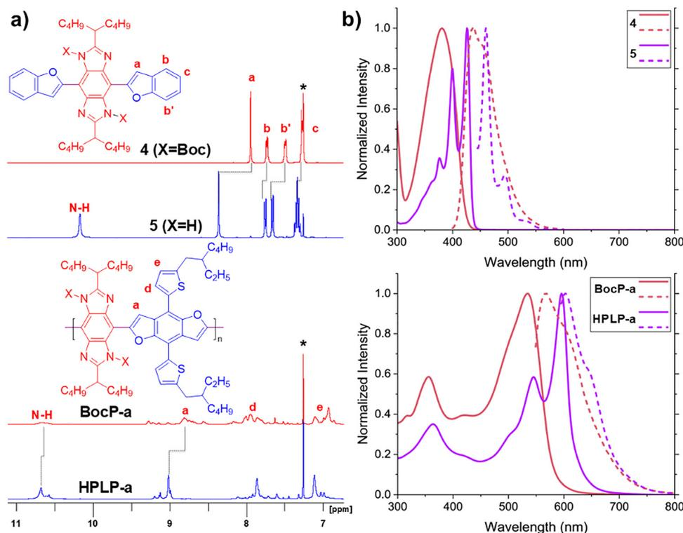
Fig. 2 (a) <sup>1</sup>H NMR spectra and of the Boc-masked species **4** and **BocP-a** ( $M_n = 7.3 \text{ kg mol}^{-1}$ ,  $D = 1.83$ ) and (b) UV-Vis (solid line) and fluorescence (dashed line) spectra of **4** and **BocP-a** ( $M_n = 16.1 \text{ kg mol}^{-1}$ ,  $D = 1.42$ ) in comparison with the corresponding unmasked derivatives.
