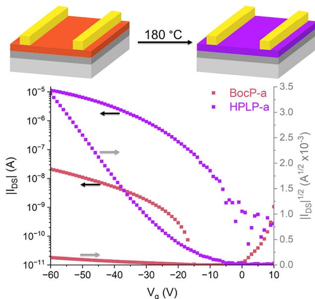
Fig. 6 (top) Schematic illustration of the thermal treatment process on the OFET device of **BocP-a**, enabling the *in situ* transformation of the active layer from **BocP-a** to **HPLP-a**; (bottom) transfer characteristics of the OFET devices before (**BocP-a**) and after (**HPLP-a**) thermal treatment at  $V_{\text{DS}} = 60$  V.
