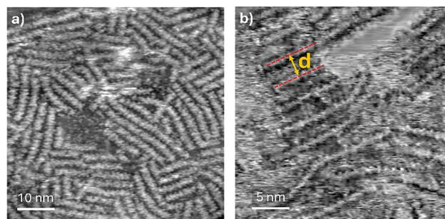
Fig. 5 (a) STM image of a high coverage area of **BocP-b** ( $M_n = 19.3$  kg mol<sup>-1</sup>,  $D = 1.50$ ) deposited by electro spray deposition on Au(111). (b) Zoomed-in image showing sections of the polymers align parallel to each other, with a distance  $d$  between them.
