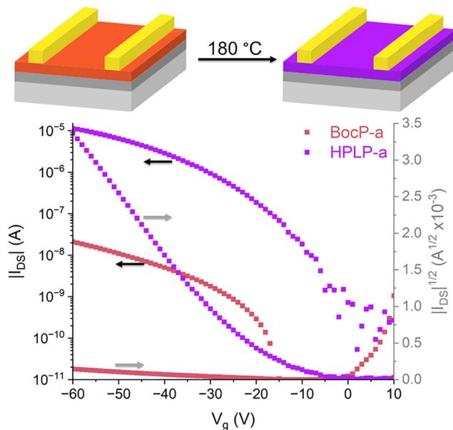
Fig. 6 (top) Schematic illustration of the thermal treatment process on the OFET device of **BocP-a**, enabling the *in situ* transformation of the active layer from **BocP-a** to **HPLP-a**; (bottom) transfer characteristics of the OFET devices before (**BocP-a**) and after (**HPLP-a**) thermal treatment at  $V_{DS} = 60$  V.
