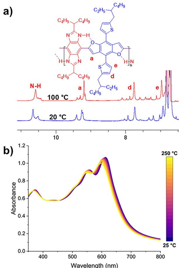
Fig. 4 (a) Variable-temperature NMR of **HPLP-a** (derived from **BocP-a**:  $M_n = 7.3$  kg mol<sup>-1</sup>,  $D = 1.83$ ) in toluene-*d*<sub>6</sub>, and (b) variable-temperature UV-Vis spectra of **HPLP-a** (from **BocP-a**:  $M_n = 16.1$  kg mol<sup>-1</sup>,  $D = 1.42$ ) in thin film.
