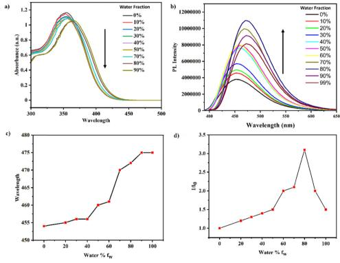
Fig. 6 (a) UV-vis absorption spectra; (b) fluorescence spectra of BPy-FL in different THF:water fraction (10<sup>-5</sup> M) solutions; (c) plot of PL wavelength vs. water fraction; and (d) plot of PL intensity vs. water fraction.
