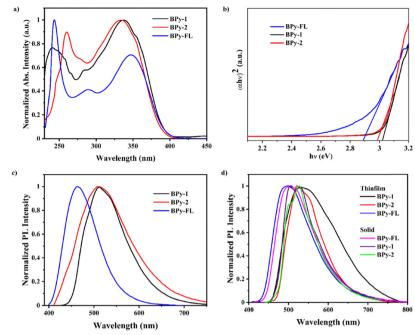
Fig. 5 (a) UV-vis spectra in dilute toluene solution (10<sup>-5</sup> M); (b) diffuse reflectance spectra (DRS) measured using solid compounds; (c) PL spectra in THF  $(10^{-5} \text{ M})$ ; and (d) thin film and solid PL.
