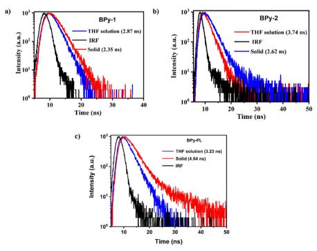
Fig. 7 Time-resolved PL decay of (a) BPy-1, (b) BPy-2, and (c) BPy-FL.
