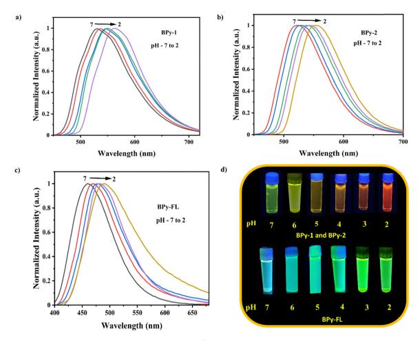
Fig. 11 Fluorescence spectra of fluorophores in THF solutions (1  $\times$  10<sup>-5</sup> M) at different pH values: (a) **BPy-1**, (b) **BPy-2** and (c) **BPy-FL**.
