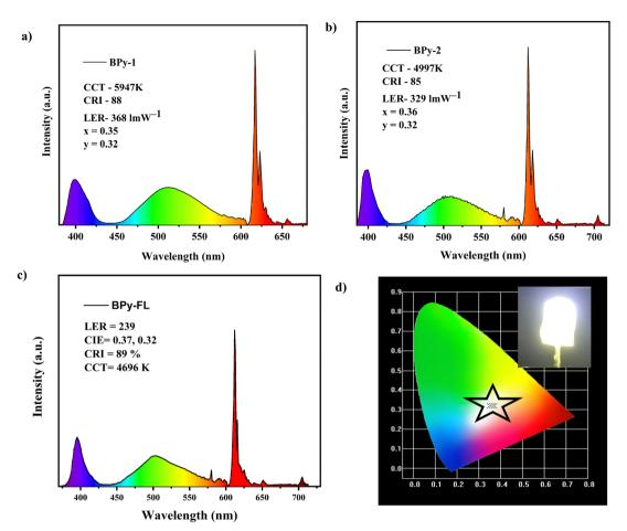
Fig. 10 PL spectra of the white LEDs fabricated using blue LED chips using the synthesized fluorophores and Eu complexes: (a) BPy-1, (b) BPy-2, and (c) BPy-FL and (d) CIE-coordinates of the fabricated white LEDs.
