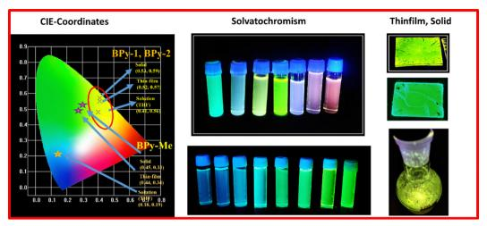
Fig. 9 CIE-coordinates of the fluorophores (solution, thin film, and solid), digital images of the fluorophores under UV-light (365 nm) in different solvents (nonpolar to polar), thin film and solid form.
