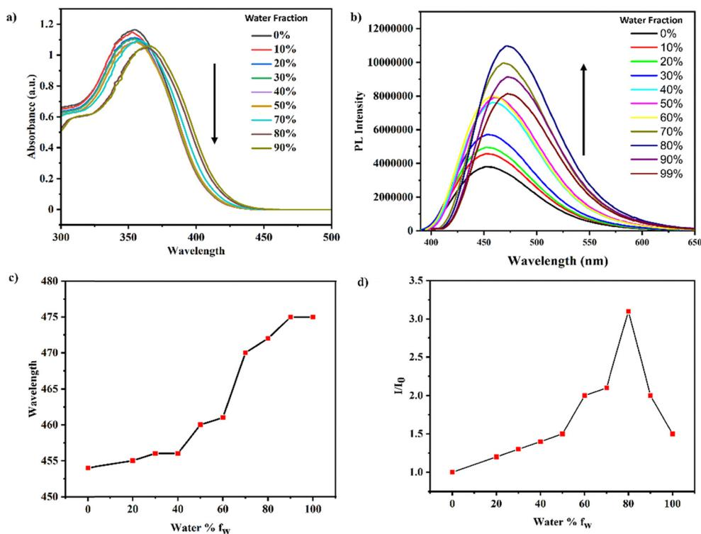
Fig. 6 (a) UV-vis absorption spectra; (b) fluorescence spectra of BPy-FL in different THF:water fraction ( $10^{-5}$  M) solutions; (c) plot of PL wavelength vs. water fraction; and (d) plot of PL intensity vs. water fraction.
