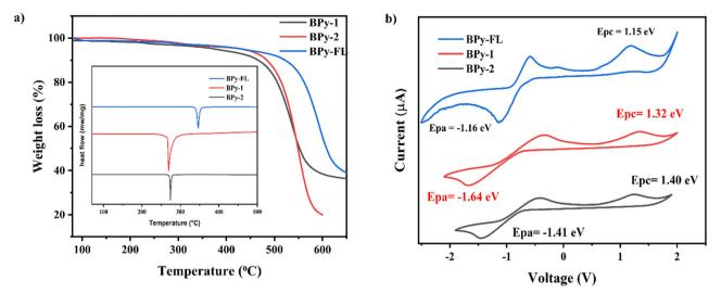
(a) TGA and DSC curves of the fluorophores under the nitrogen atmosphere and (b) cyclic voltammetry (CV) of the fluorophores
