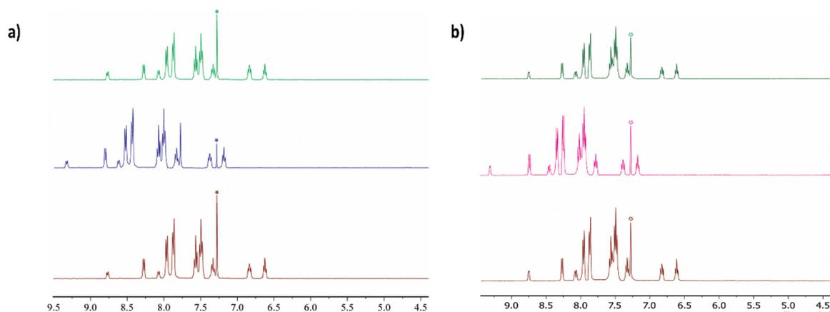
Fig. 12  $^1\text{H}$  NMR spectra of the fluorophores in  $\text{CDCl}_3$  before the addition of TFA (lower spectra) and after the addition of 2 equiv. of TFA (middle) and 10 equiv. of TEA (upper): (a) **BPY-1** (b) **BPY-2**.
