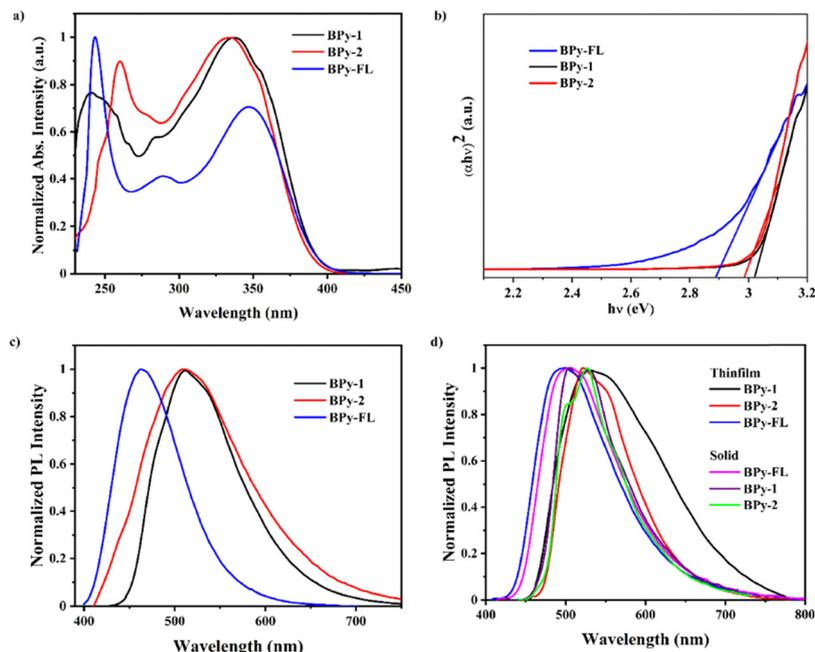
Fig. 5 (a) UV-vis spectra in dilute toluene solution ( $10^{-5}$  M); (b) diffuse reflectance spectra (DRS) measured using solid compounds; (c) PL spectra in THF ( $10^{-5}$  M); and (d) thin film and solid PL.
