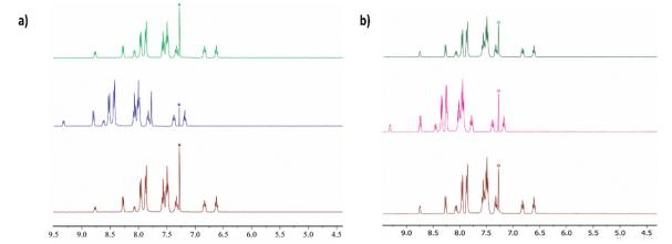
Fig. 12 <sup>1</sup>H NMR spectra of the fluorophores in CDCl<sub>3</sub> before the addition of TFA (lower spectra) and after the addition of 2 equiv. of TFA (middle) and 10 equiv. of TEA (upper): (a) BPy-1 (b) BPy-2.
