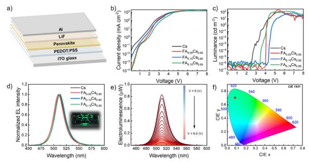
Fig. 9 Performance of fabricated Cs,  $FA_{0.05}Cs_{0.95}$ ,  $FA_{0.10}Cs_{0.90}$ , and  $FA_{0.15}Cs_{0.85}$  LEDs showing their (a) simple device architecture, (b) J-V curves, (c) luminance (L-V) curves, and (d) electroluminescence with device under operation (visual image of the device emitting green light, inset). (e) Electroluminescence at varying voltages and (f) the CIE color coordinates and the operating LED showing the green emission for FA<sub>0.05</sub>Cs<sub>0.95</sub> LED.
