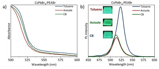
Fig. 2 Optical characterization of optimized CsPbBr<sub>3</sub> perovskite films. (a) Absorbance and (b) PL spectra measurements of CsPbBr<sub>3</sub>:PEABr films treated with toluene, anisole, and CB.
