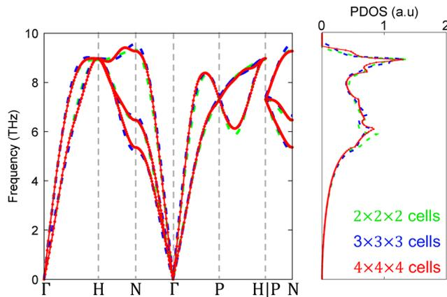
Fig. 4 Phonon dispersion and phonon density of states (DOS) for bcc Fe, calculated for supercell sizes of  $2 \times 2 \times 2$ ,  $3 \times 3 \times 3$ , and  $4 \times 4 \times 4$  by combining VASP and Phonopy codes.
