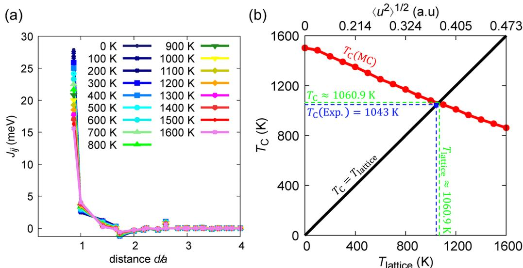
Fig. 5 (a) Temperature dependence of magnetic exchange coupling constants  $J_{ij}$  for Fe–Fe pairs in bcc Fe, including the effects of thermal lattice vibration ( $T_{\text{lattice}}$ ) by using the SPR-KKR code for the DLM state. (b) Curie temperature of bcc Fe as determined by Monte Carlo simulations, shown as a function of the amplitude of thermal lattice vibration effects (root mean square of lattice displacement,  $\langle u^2 \rangle^{1/2}$  or  $T_{\text{lattice}}$ ).
