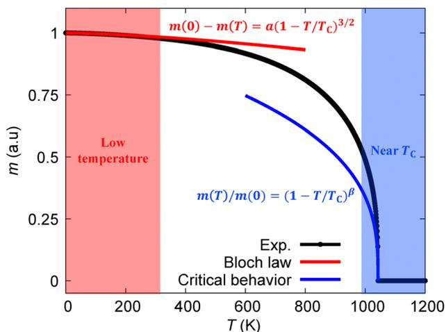
Fig. 1 Normalized spontaneous magnetization of body-centered cubic (bcc) Fe in experimental work as Kuz'min formula<sup>15</sup> (black color), Bloch law at low temperature (red color), and critical exponential or Landau theory near Curie temperature (blue color).
