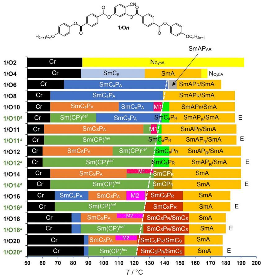
Fig. 3 Bar diagram of compounds **1/On** showing the development of the LC phases on cooling and depending on chain length (see Table 2 for abbreviations and numerical values). <sup>a</sup> E indicates transitions after treatment with few cycles of an alternating electric field; the dashed white line indicates the approximate chain-length dependence of the Curie temperatures of the paraelectric–ferroelectric transition.
