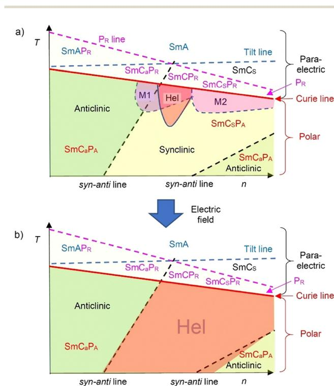
Fig. 18 Sketch of the development of tilt, polar order and helicity in the smectic LC phases of the bent-core molecules 1/On depending on temperature and alkyl chain length ( $n = 8-20$ ): (a) in the pristine material and (b) after applying a short AC sequence; Hel = heliconical Sm(CP)<sup>hel</sup> phase, for other abbreviations, see Table 2.
