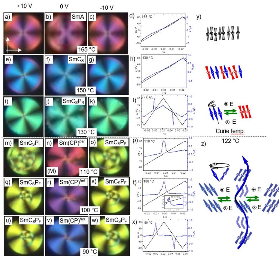
Fig. 13 (a)–(x) Switching in the smectic phases of compound **1/O20** (6  $\mu\text{m}$  non-coated ITO cell). The three left columns show circular domain as observed by POM upon cooling, from left to right at +10 V, after switching off the applied voltage, and at  $-10$  V; the right column show the corresponding polarization current curves (160  $V_{pp}$ , 10 Hz); (y) and (z) show sketches of molecular reorganization for the distinct switching processes.
