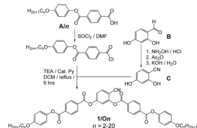
Scheme 1 Synthetic route to the bent-core mesogens **1/On**.
