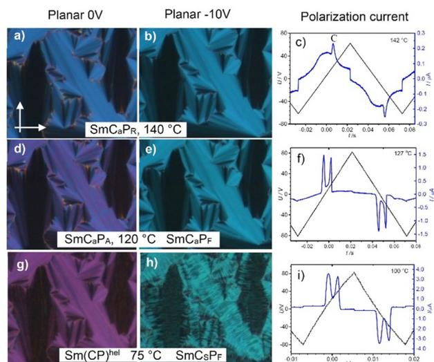
Fig. 7 Optical micrographs of the POM textures observed for the different LC phases of compound **1/O10** in a PI coated 6  $\mu\text{m}$  ITO cell in planar alignment, (a), (d) and (g) without applied electric field, (b), (e) and (h) after application of 6 V DC field, and (c), (f) and (i) polarization current response curves in the same cell at the indicated temperatures; in c) C indicates the conductivity peak; all data were recorded on cooling.
