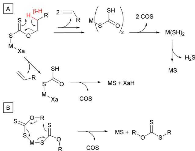
**Scheme 1** (A) Chugaev-like degradation pathway for metal xanthates forming the metal sulfide and COS, alkene and xanthic acid side products. (B) Degradation pathway for xanthates proposed by A. Piquette, yielding a purely organic xanthate *via* an alkyl transfer.<sup>2</sup>
