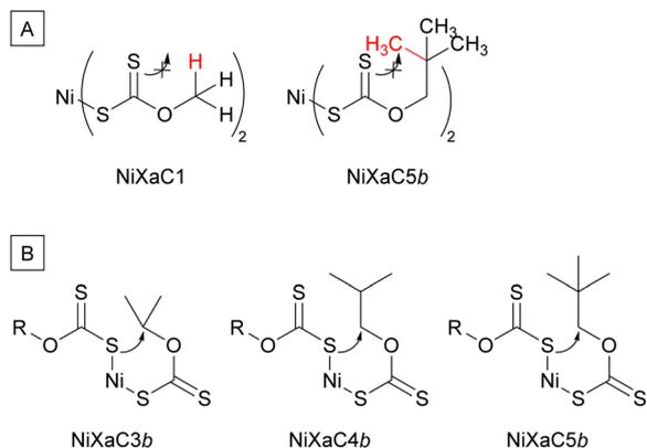
**Scheme 3** (A) Synthesized compounds without  $\beta$ -hydrogen (nickel methyl- and neopentyl xanthate). (B) Xanthates with branched alkyl substituents (NiXaC3b, NiXaC4b and NiXaC5b) investigated by pyrolysis-GC-HRMS.
