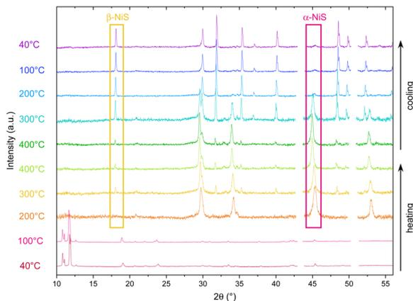
Fig. 7 XRD heating run of the precursor NiXaC4b. Heating rate:  $2\text{ }^{\circ}\text{C min}^{-1}$ , 30 minutes holding steps at  $400\text{ }^{\circ}\text{C}$  during heating and at  $40\text{ }^{\circ}\text{C}$  after cooling.
