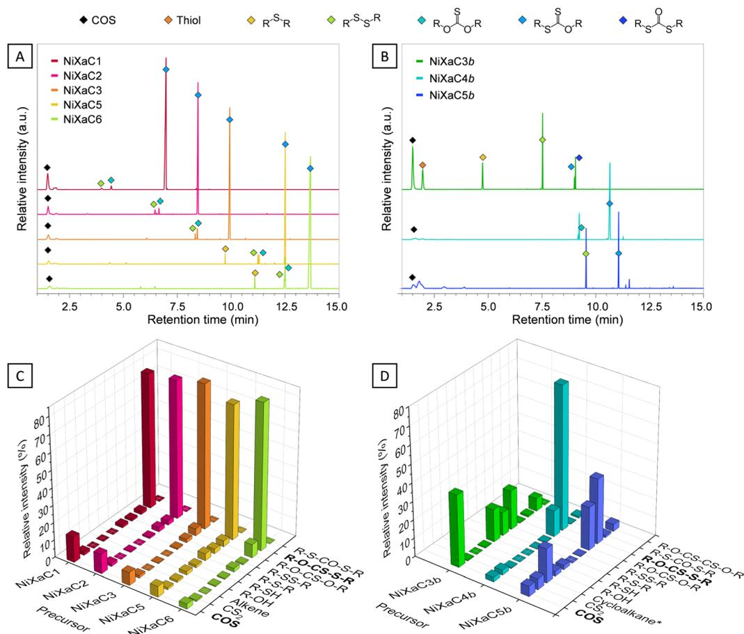
**Fig. 3** Pyrolysis-GC-MS traces for the linear (A) and branched (B) nickel xanthates with labels for the main compound peaks. Derived degradation product profiles for the linear (C) and branched (D) nickel xanthates. Cycloalkane\* (D) was found only for the NiXaC5b precursor.
