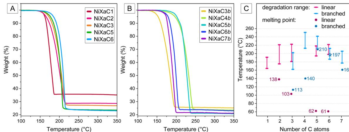
**Fig. 2** TGA curves for the nickel xanthate precursors with linear (A) or branched side chains (B). Onset was determined by the tangent method. (C) Decomposition temperature ranges and melting temperatures for nickel xanthate precursors with different linear and branched side chains. Pink: linear side chains, blue: branched side chains.
