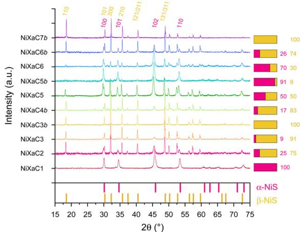
**Fig. 9** Powder XRD measurements of the different NiXa precursors after sintering at 400 °C, N<sub>2</sub>; with references for  $\alpha$ -NiS and  $\beta$ -NiS given below. Right: Ratio of  $\alpha$ -NiS and  $\beta$ -NiS estimated from the intensities of the major reflections of the respective phases ( $\alpha$ -NiS: (102), 45.9°  $2\theta$ ,  $\beta$ -NiS: (300), 32.2°  $2\theta$ /(313), 48.8°  $2\theta$ ).
