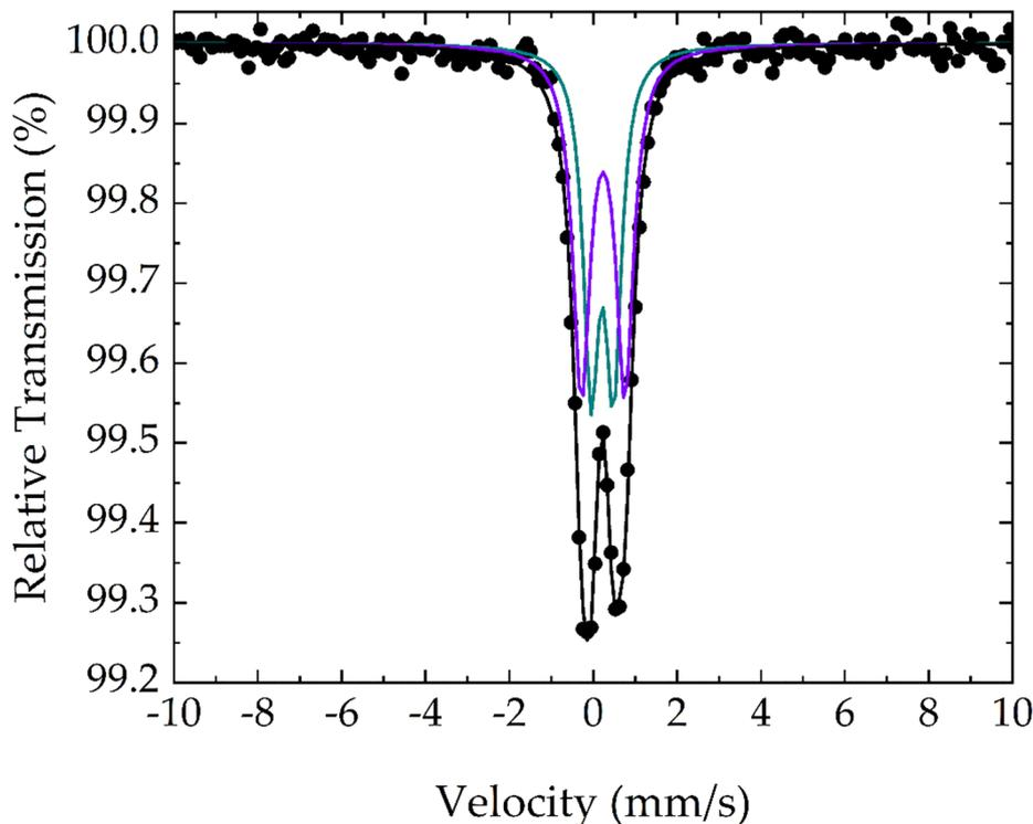
Fig. 5  $^{57}\text{Fe}$  Mössbauer fitted spectrum of the AM-NHD precursor collected at room temperature. Points represent the experimental data and the coloured lines the components used to fit the spectrum.
