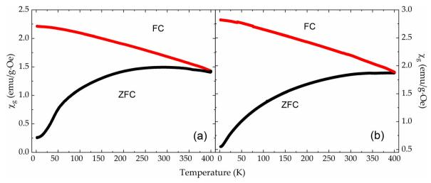
Fig. 9 Magnetic susceptibility vs. temperature measurements of the NHD-700C,30m (a) and NHD-700C,4h (b) samples conducted under an applied field of 99 Oe
