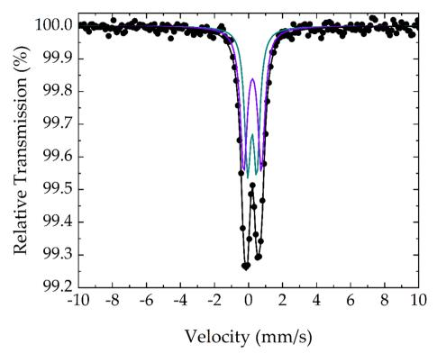
Fig. 5 57Fe Mössbauer fitted spectrum of the AM-NHD precursor collected at room temperature. Points represent the experimental data and the coloured lines the components used to fit the spectrum.
