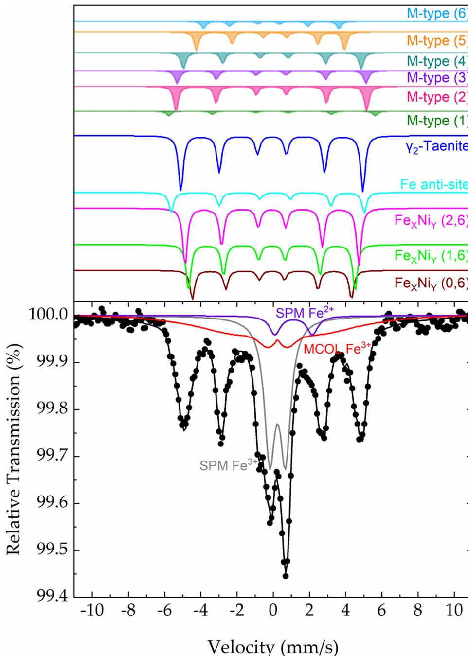
Fig. 6  $^{57}\text{Fe}$  Mössbauer fitted spectrum of the NHD-700C,30m sample collected at room temperature. Points represent the experimental data and the coloured lines the components used to fit the spectrum, with some of their base-lines shifted higher than 100% relative transmission to improve the clarity of this multicomponent fitting.
