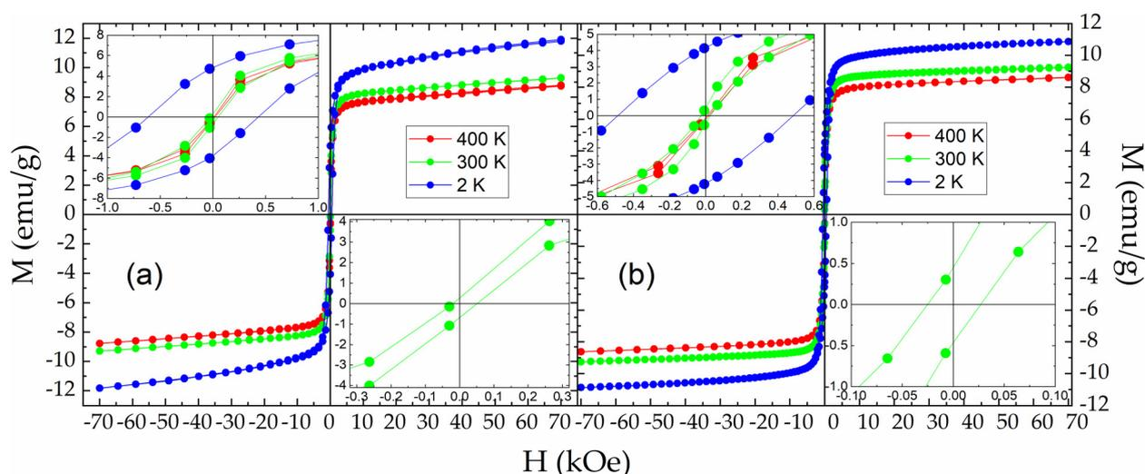
Fig. 8 Magnetization *vs.* applied magnetic field isothermal loops of the NHD-700C,30m (a) and En-NHD-700C,4h (b) samples measured at different temperatures indicated by different colours. The insets in each set of measurements show the details of the loops' characteristics around zero applied magnetic field for all temperatures (upper left) and with even more detail for the 300 K loop (lower right).
