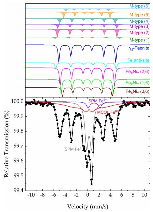
Fig. 6 57Fe Mössbauer fitted spectrum of the NHD-700C,30m sample collected at room temperature. Points represent the experimental data and the coloured lines the components used to fit the spectrum, with some of their base-lines shifted higher than 100% relative transmission to improve the clarity of this multicomponent fitting
