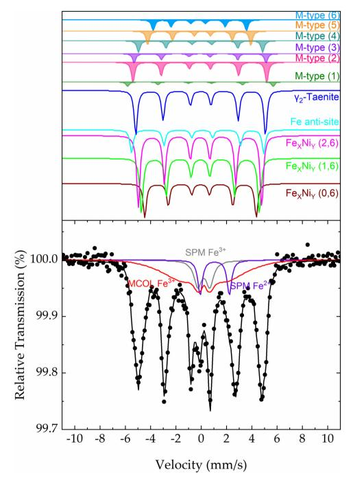
Fig. 7 57Fe Mössbauer fitted spectrum of the NHD-700C,4h sample collected at room temperature. Points represent the experimental data and the coloured lines the components used to fit the spectrum, with some of their base-lines shifted higher than 100% relative transmission to improve the clarity of this multicomponent fitting.
