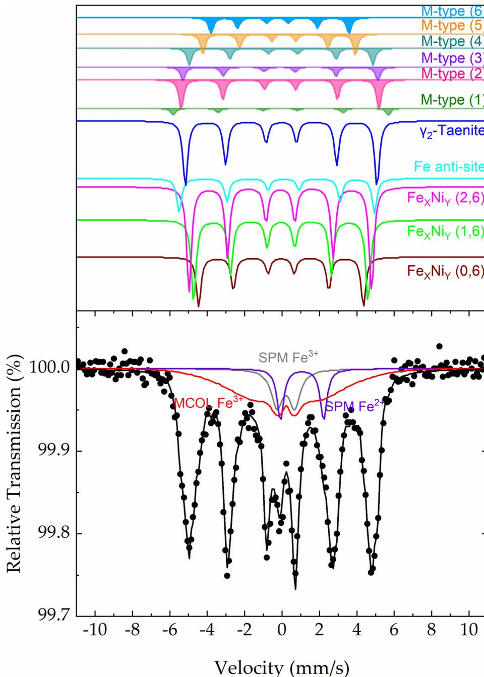
Fig. 7  $^{57}\text{Fe}$  Mössbauer fitted spectrum of the NHD-700C,4h sample collected at room temperature. Points represent the experimental data and the coloured lines the components used to fit the spectrum, with some of their base-lines shifted higher than 100% relative transmission to improve the clarity of this multicomponent fitting.
