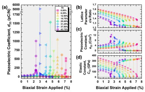
Fig. 3 Plots of (a) piezoelectric coefficients,  $d_{33}$ , (b) lattice parameter c/a ratio, (c) piezoelectric constant,  $e_{33}$ , and (d) elastic constant,  $C_{33}$ , versus biaxial strain applied for different Sc fraction, x, for Al<sub>1-x</sub>Sc<sub>x</sub>N SQS supercells. The black horizontal dashed lines represent the abscissa.
