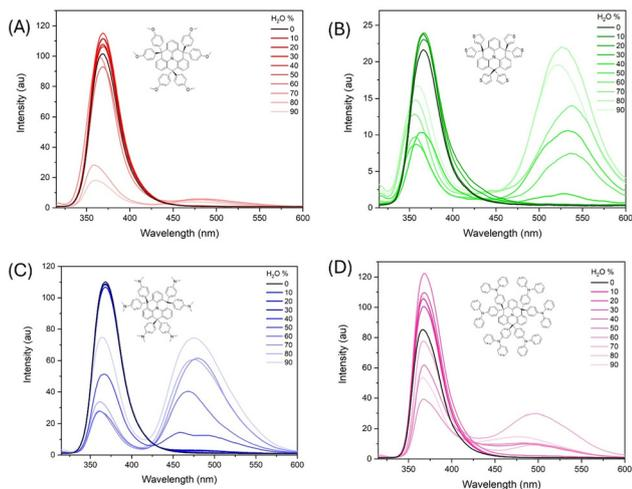
Fig. 5 Fluorescence intensity of **FTPA-OMe** (A), **FTPA-Thio** (B), **FTPA-NMe<sub>2</sub>** (C), and **FTPA-TPA** (D) in THF/water mixtures with increasing water fractions ( $f_w$ ) from 0% to 90%, performed at constant concentration of  $1 \times 10^{-5}$  M ( $\lambda_{\text{ex}} = 310$  nm).
