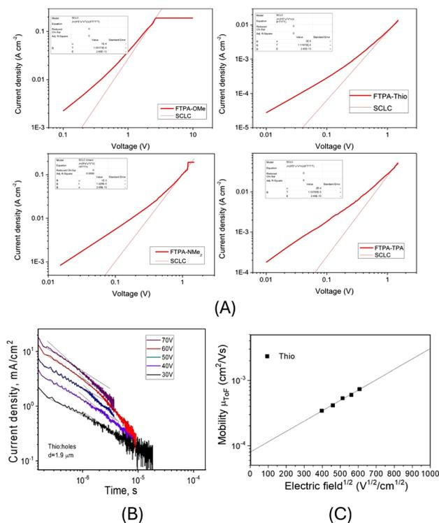
Fig. 8 (A)  $J$ – $V$  curves with space-charge-limited current mobility fitting. (B) TOF data and (C) electric field dependence of hole mobility in vacuum-deposited film of **FTP-Thio**.
