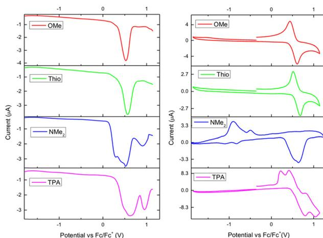
Fig. 7 Electrochemical analysis of all compounds (SWV left, CV right). All measurements were conducted at  $5 \times 10^{-4}$  M<sup>-1</sup> in CH<sub>2</sub>Cl<sub>2</sub> with 0.1 M TBAPF<sub>6</sub> as the supporting electrolyte and ferrocene as an external standard.
