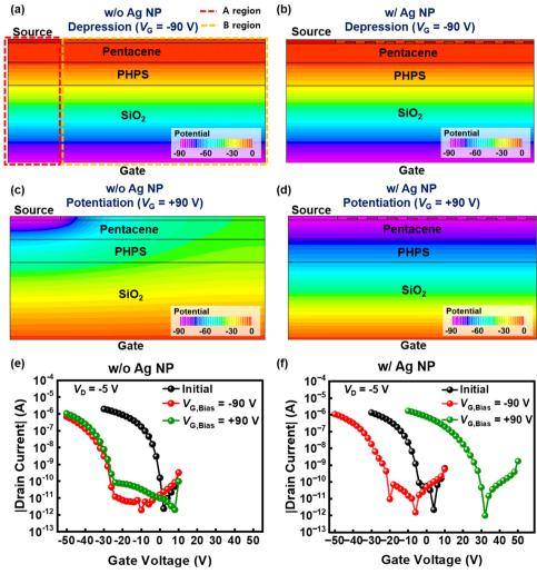
Fig. 2 Simulated potential distribution results without and with Aq NPs during the (a) and (b) write (depression) and (c), (d) erase (potentiation) operations. Transfer curves of the devices (e) without and (f) with Ag NPs after writing (red line) and erasing (green line), with the black lines representing the initial transfer curves.
