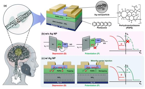
Fig. 1 (a) Schematic of charge-trapping-based OSTs with metal NPs for electrically writable (depression; D) and erasable (potentiation; P) multi-memory states in neuromorphic computing. (b) Challenges in electrical erase operations (P) of charge-trapping-based OSTs with oligomeric semiconductors. (c) Realization of electrically writable (D) and erasable (P) multi-memory states by introducing metal NPs on top of the OSC layer.
