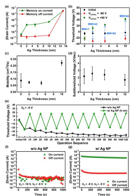
Fig. 3 (a) Graph of the memory on-current and memory off-current, (b) memory window, (c) mobility values, and (d) subthreshold voltage values of the OSTs as a function of Aq NP thickness. (e) Ten cycles of writing and erasing processes. Retention characteristics of OSTs (f) without and (g) with Aq NPs.
