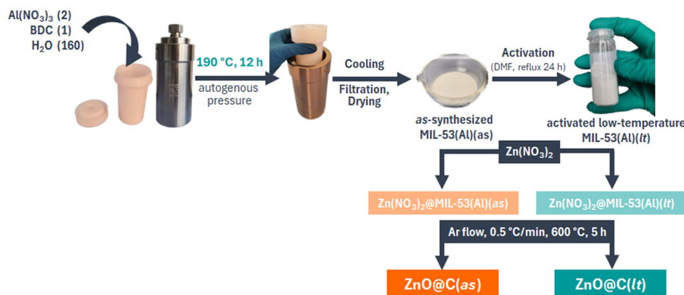
Scheme 1 Synthesis route for the ZnO@C samples derived from MIL-53(Al) metal–organic framework.
