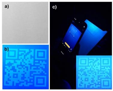
Fig. 6 Aqueous solution 25 mg  $mL^{-1}$  of N-CDs inkjet printed on Bristol drawing paper, (a) shown under daylight and (b) under 365 nm UV light. (c) Smartphone read out of the printed QR code after one year of storage in the dark at room temperature. Inset of the QR emission after one year of storage.
