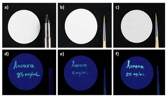
Fig. 5 Aqueous solution 25 mg mL<sup>-1</sup> of N-CDs handwritten on Whatman<sup>®</sup> filter paper, shown (a) under daylight and (d) under 365 nm UV light. Aqueous solution 5 mg mL<sup>-1</sup> of N-CDs brushed on Whatman<sup>®</sup> filter paper, shown (b) under daylight and (e) under 365 nm UV light. Aqueous solution 25 mg mL<sup>-1</sup> of N-CDs brushed on Whatman® filter paper, shown (c) under daylight and (f) under 365 nm UV light.
