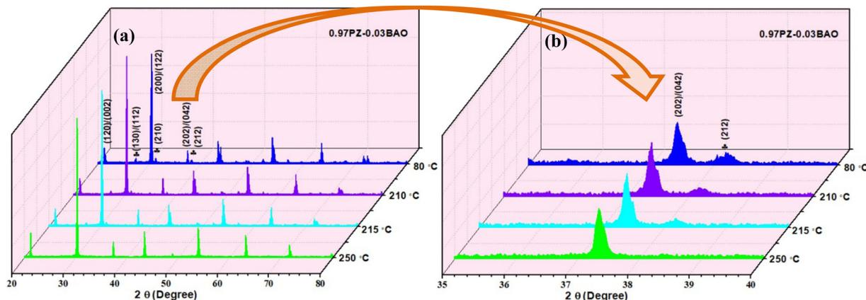
Fig. 3 (a) XRD patterns of the  $(1-x)\text{PZ}-x\text{BA}$  ceramics for  $x = 0.03$  measured at the temperatures of 80 °C, 210 °C, 215 °C and 250 °C. The peaks marked with “\*” indicate the 1/4 superlattice reflections. (b) Enlarged view of the perovskite lattice peak (202)/(042) and the superlattice reflection (212).
