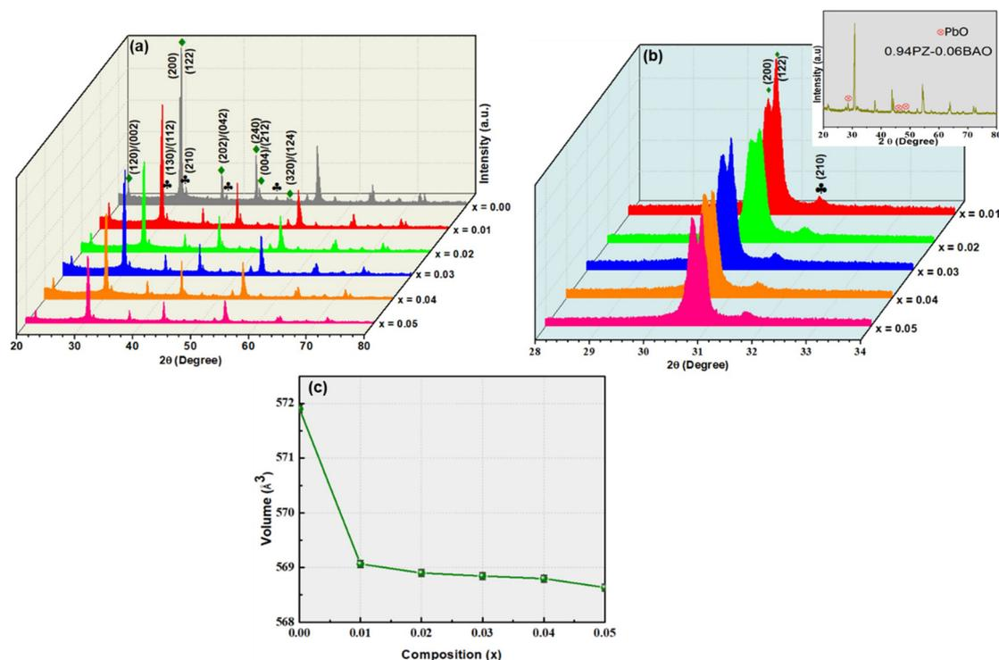
**Fig. 2** (a) Room temperature XRD patterns of the  $(1-x)\text{PZ}-x\text{BA}$  ceramics for  $0.00 \leq x \leq 0.05$ . (b) Enlarged view of the (200)/(122) peaks at  $2\theta = 31^{\circ}$  and the superlattice (210) reflection at  $2\theta = 31.9^{\circ}$ . The inset shows the XRD pattern for  $x = 0.06$  with the impurity peaks marked. (c) Variation of the unit cell volume as a function of composition  $x$ .
