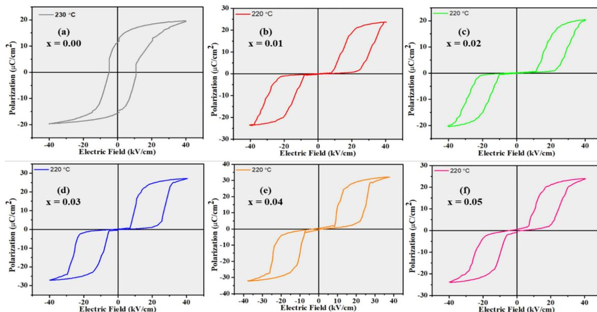
Fig. 7 (a)–(f) Polarization–electric field ( $P$ – $E$ ) relationships of the  $(1 - x)\text{PZ}-x\text{BA}$  ceramics ( $x = 0.0, 0.01, 0.02, 0.03, 0.04$  and  $0.05$ ) measured under electric fields of  $\pm 40 \text{ kV cm}^{-1}$  at a 10 Hz frequency.
