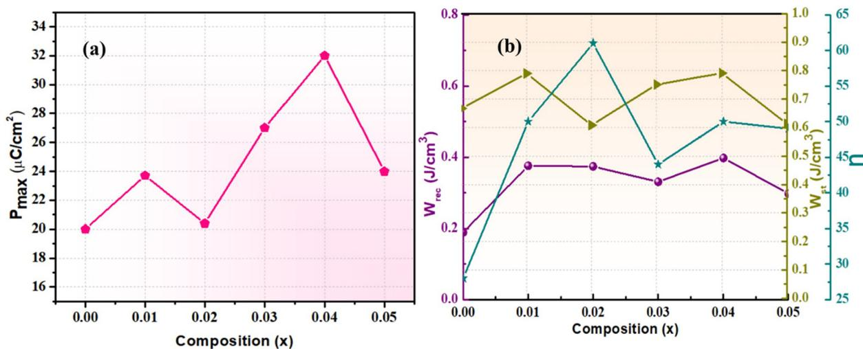
Fig. 8 (a) Maximum polarization ( $P_{\max}$ ) as a function of composition for the  $(1-x)\text{PZ}-x\text{BA}$  ( $0.00 \leq x \leq 0.05$ ) solid solution measured at 220 °C. (b) Variations of the  $W_{\text{rec}}$ ,  $W_{\text{st}}$  and  $\eta$  values as a function of composition.
