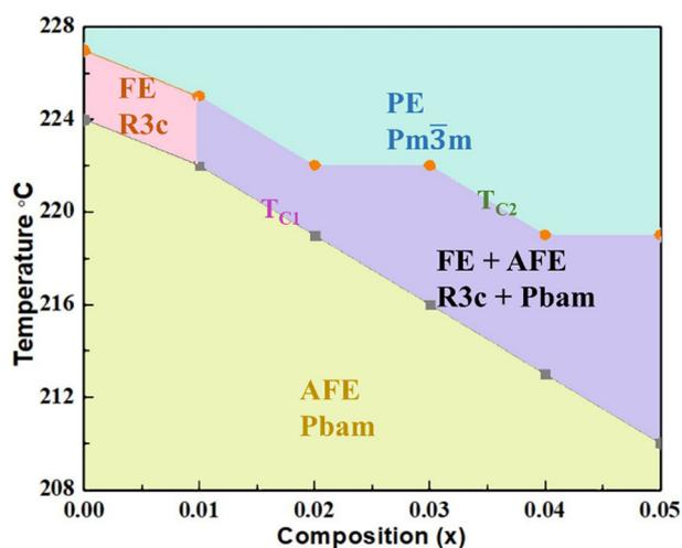
Fig. 9 Phase diagram of the  $(1-x)\text{PZ}-x\text{BA}$  ( $0.00 \leq x \leq 0.05$ ) solid solution in terms of temperature and composition  $x$ , which delimits the various phase areas and transformations between them.
