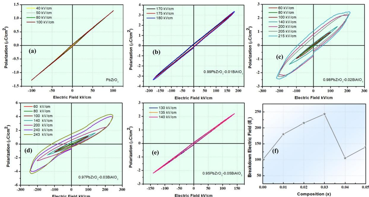
Fig. 6 (a)–(e) Room temperature polarization–electric field relationships of the  $(1 - x)\text{PZ}-x\text{BA}$  ceramics measured at a frequency of 10 Hz. (f) Maximum applied field (or breakdown) electric field ( $E_b$ ) as a function of composition  $x$ .
