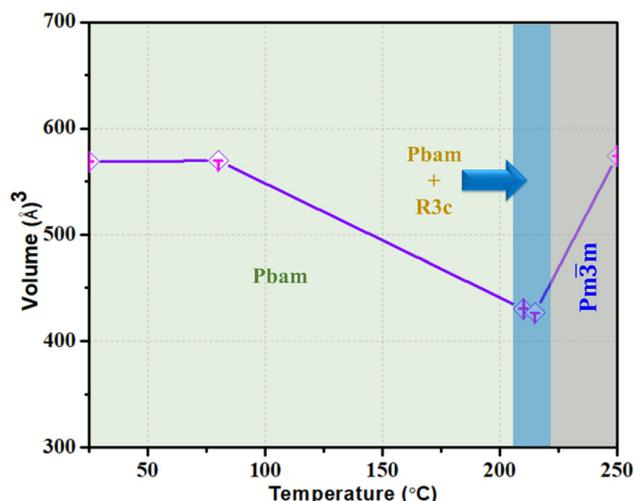
Fig. 5 Variation of the unit cell volume as a function of temperature for the 0.97PZ–0.03BA ceramics, with the temperature ranges of the *Pbam* phase, the mixed *Pbam* and *R3c* phases, and the *Pm* $\bar{3}$ *m* phase indicated.
