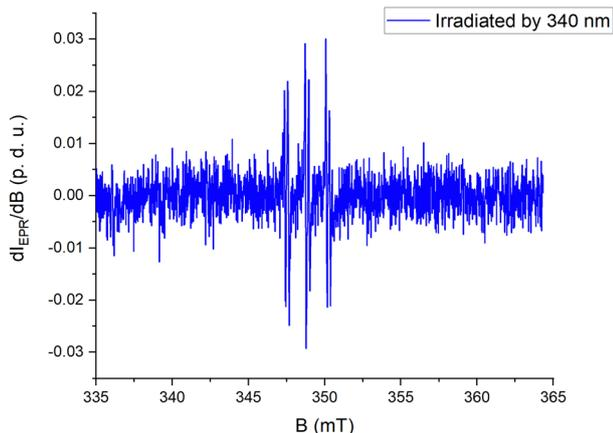
Fig. 4 EPR spectrum (X-band) of the trapped radical species between irradiated AH5 and the spin trap agent in acetonitrile. Concentrations were set to  $c(\text{AH5}) = 10 \text{ mM}$  and  $c(\text{N-t-butyl-}\alpha\text{-phenylnitron}) = 45 \text{ mM}$ . The EPR spectrum was centered at  $g_{\text{iso}} = 2.0065$ . The hyperfine splitting structure comes from a  $(1 \times ^{14}\text{N}) = 1.35 \text{ mT}$  and a  $(1 \times ^1\text{H}) = 0.22 \text{ mT}$ .
