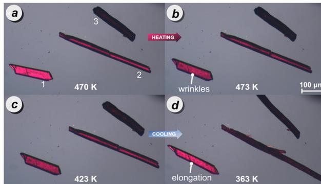
Fig. 2 Hot stage microscopy of PDI-C<sub>6</sub> crystals during the heating cycle: (a) phase I at 470 K, (b) transition from phase I to phase II at 473 K; and during cooling cycle: (c) phase II at 423 K, (d) transition from phase II to phase I at 363 K, reshaping the crystals. Additional images are provided in Fig. S18 and S19 of the ESI†
