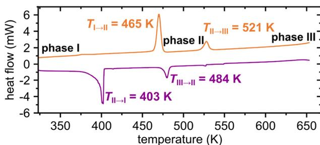
Fig. 1 Differential scanning calorimetry (DSC) thermogram of PDI-C<sub>6</sub> in the heating (top) and cooling (bottom) cycles. Temperatures of phase transitions are indicated.
