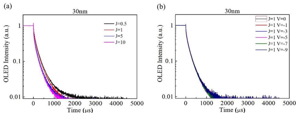
Fig. 9 The transient electroluminescence of the 15% **4SpAc35CzPy**: **o-DiCzBz** TADF-OLED. Delayed luminescence was observed after cutting off the power supply: (a) TrEL with different driving currents. (b) TrEL with different reverse-bias electrical voltages.
