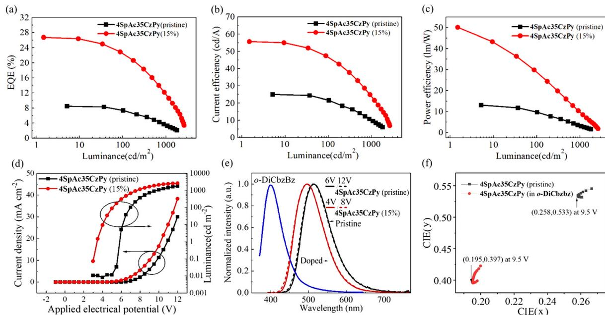
Fig. 8 Spectral and EL properties of the OLEDs, using 15% **4SpAc35CzPy** doped or the non-doped **4SpAc35CzPy** as the EML: (a) EQE vs. luminescence; (b) CE vs. luminescence; (c) PE vs. luminescence; (d) current density vs. applied electrical potential; (e) EL spectrum; (f) CIE ( $x,y$ ).
