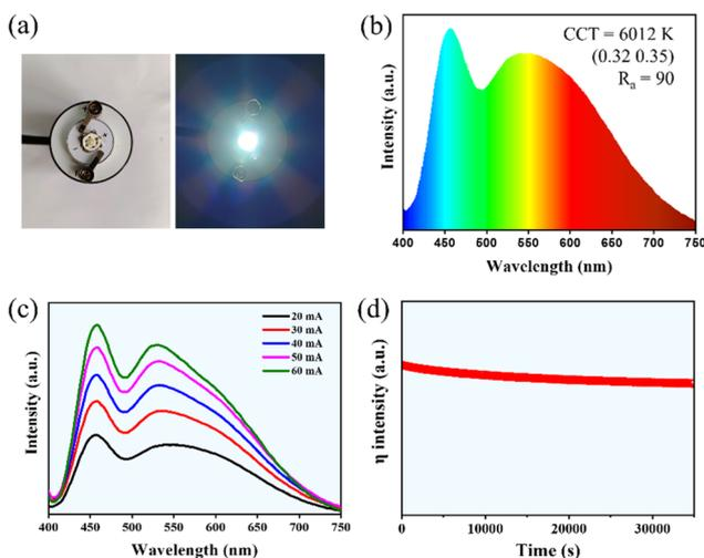
**Fig. 6** Performance of the WLED using  $[\text{FBZPA}]_4\text{Cu}_5\text{Br}_{13}$  crystals as a yellow-emitting phosphor. (a) Images of the fabricated white LED, including its operation at a drive current of 20 mA. (b) Electroluminescence (EL) spectrum at a drive current of 20 mA. (c) EL spectra under varying drive currents from 20 to 60 mA. (d) Time-dependent luminescence efficiency during continuous operation.
