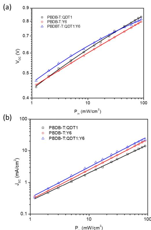
Fig. 4 Dependence of (a)  $V_{OC}$  and (b)  $J_{SC}$  with  $P_{in}$  for optimized binary (PBDB-T:**QDT1** and PBDB-T:Y6) and ternary (PBDB-T:**QDT1**:Y6) OSCs.
