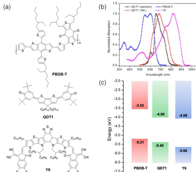
Fig. 1 (a) Chemical structures of PBDB-T, QDT1, and Y6. (b) UV-Vis-NIR spectra of QDT1 in solution, QDT1 in thin film, PBDB-T in thin film, and Y6 in thin film. (c) Schematic energy level diagrams of materials used in photovoltaic devices.
