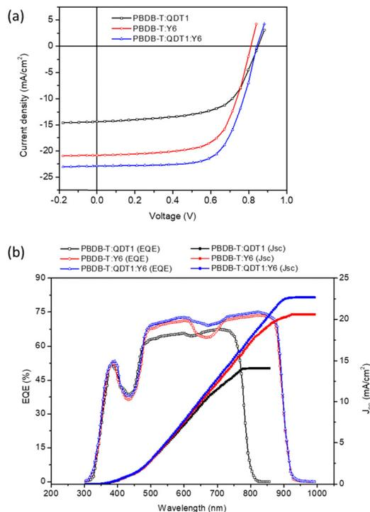
Fig. 2 (a) *J–V* characteristics under 1 sun condition (AM1.5G, 100 mW cm<sup>-2</sup>), (b) EQE spectra of the optimized binary (PBDB-T:QDT1 and PBDB-T:Y6) and ternary PBDB-T:QDT1:Y6 OSCs.
