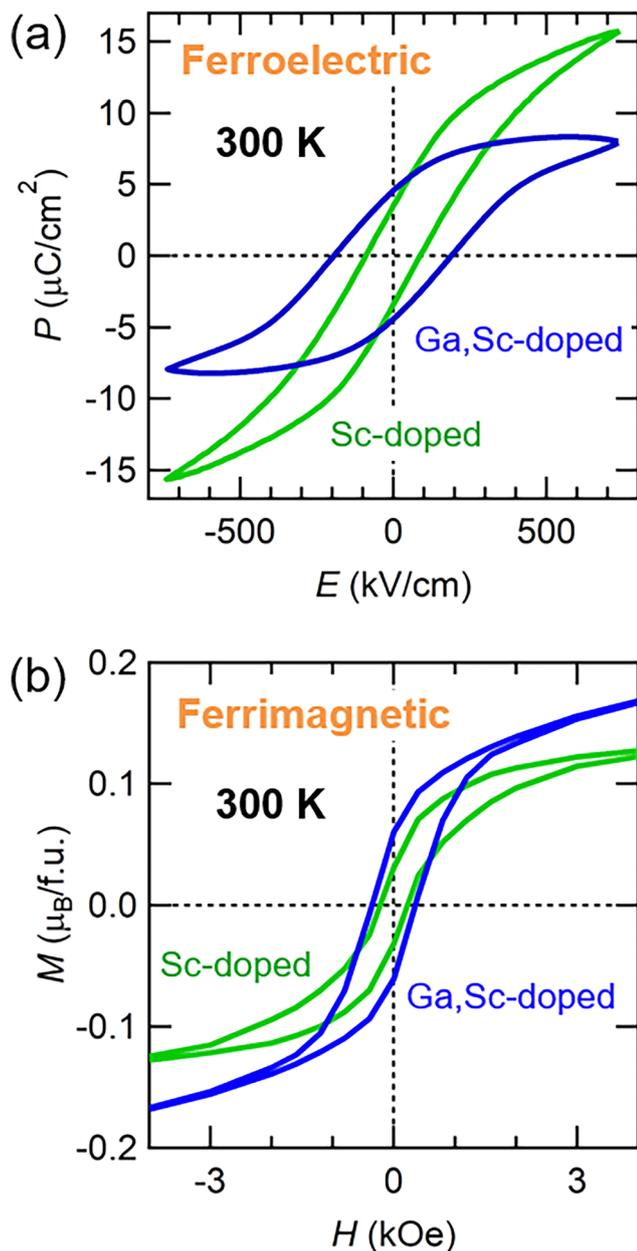
Fig. 6 (a) Polarization ( $P$ ) versus electric field ( $E$ ) and (b) magnetization ( $M$ ) versus magnetic field ( $H$ ) curves for the Sc-doped and Ga,Sc-codoped  $\epsilon$ - $\text{Fe}_2\text{O}_3$  films at 300 K.
