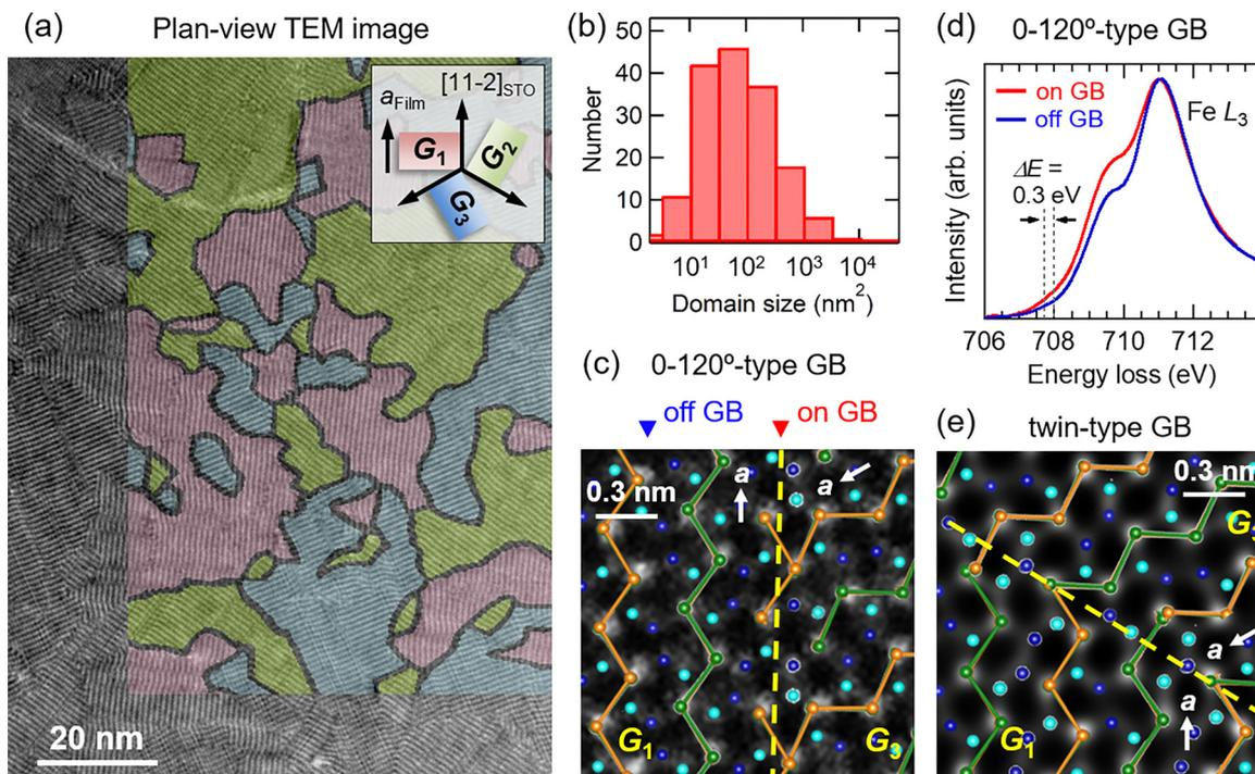
Fig. 2 (a) Plan-view TEM image. (b) A histogram of the grain size. (c) Plan-view STEM image and (d) on- and off-GB Fe  $L_3$ -edge EELS spectra near the 0–120°-type grain boundaries (GBs). (e) Plan-view STEM image near twin-type GBs for the Ga-doped  $\epsilon$ - $\text{Fe}_2\text{O}_3$  film.
