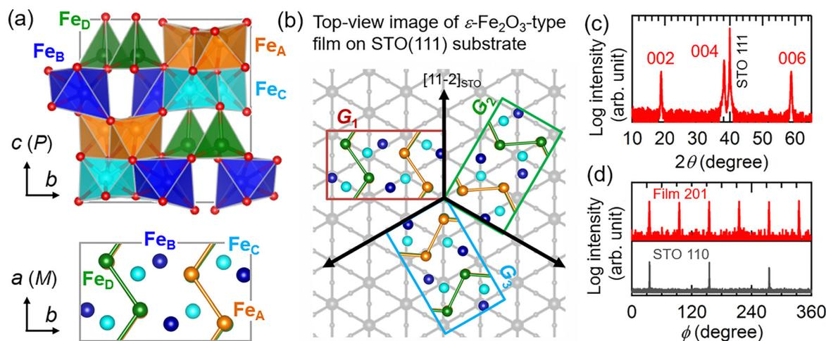
Fig. 1 (a) Crystal structures of  $\epsilon$ -Fe<sub>2</sub>O<sub>3</sub> and (b) top-view schematic of the  $\epsilon$ -Fe<sub>2</sub>O<sub>3</sub>-related oxide film grown on the STO(111) substrate. (c)  $2\theta$ - $\theta$  X-ray diffraction pattern and (d)  $\phi$ -scan of the Ga-doped  $\epsilon$ -Fe<sub>2</sub>O<sub>3</sub> film.
