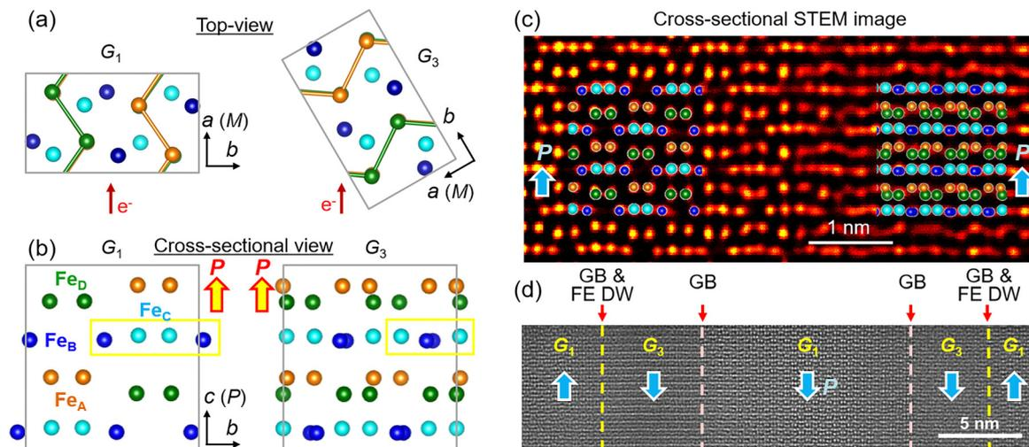
Fig. 3 (a) Top-view and (b) cross-sectional images of  $\epsilon$ - $\text{Fe}_2\text{O}_3$ . (c) and (d) Cross-sectional HAADF-STEM images of the Ga-doped  $\epsilon$ - $\text{Fe}_2\text{O}_3$  film.
