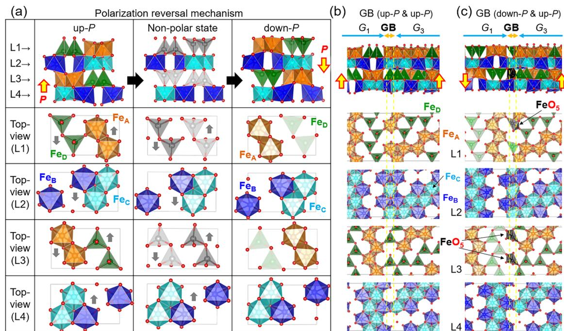
Fig. 4 (a)  $P$ -reversal mechanism in  $\epsilon$ - $\text{Fe}_2\text{O}_3$ . (b)  $0$ - $120^\circ$ -type GB structure between the up- $P$   $G_1$  and up- $P$   $G_3$  domains. (c) Expected GB structure after  $P$  reversal in the  $G_1$  domain.
