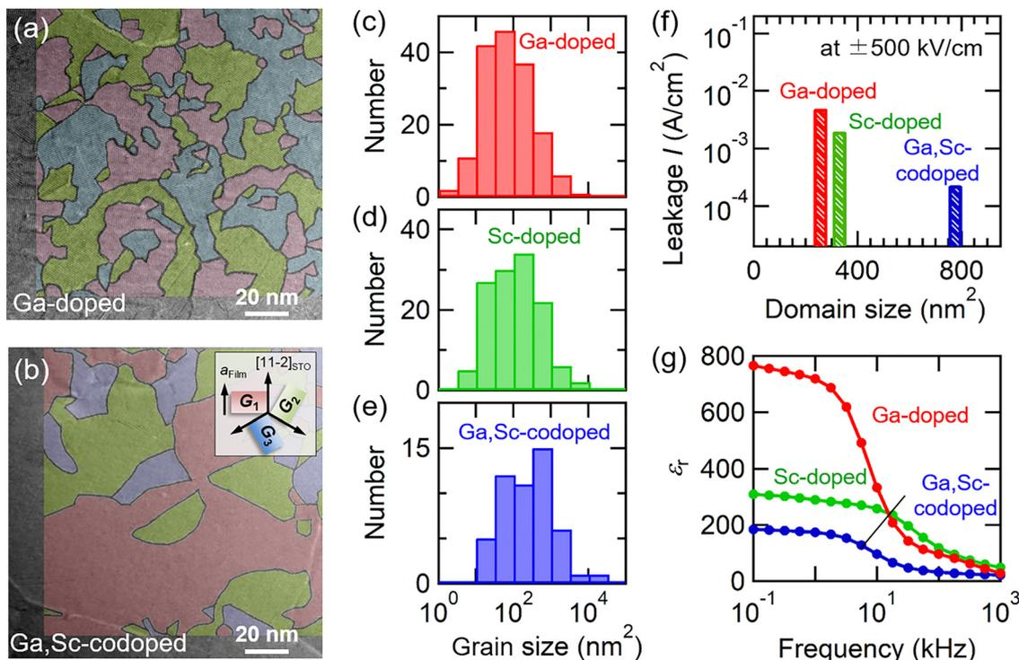
Fig. 5 Plan-view TEM images and histograms of the grain size for the (a) and (c) Ga-doped, (d) Sc-doped, and (b) and (e) Ga,Sc-codoped  $\epsilon$ - $\text{Fe}_2\text{O}_3$  films. (f) Leakage current and (g) permittivity of the films at 300 K.
