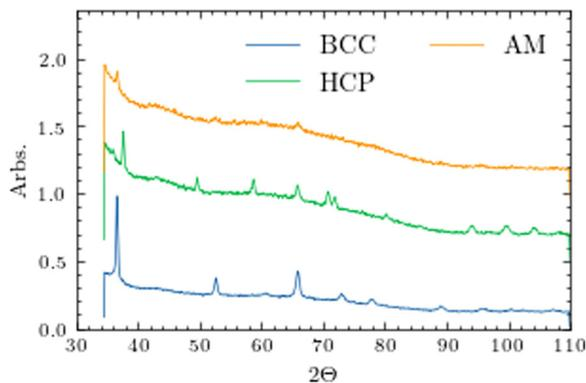
Fig. 3 X-Ray diffraction patterns for the primarily BCC (blue), HCP (green), and amorphous (AM – yellow) phases. Data was smoothed with a 10-point simple moving average to improve clarity before normalization. (Cu K $\alpha$  radiation) The large dome-like background present in each scan is presumed to be an underlying amorphous phase limiting our ability to do quantitative analysis.
