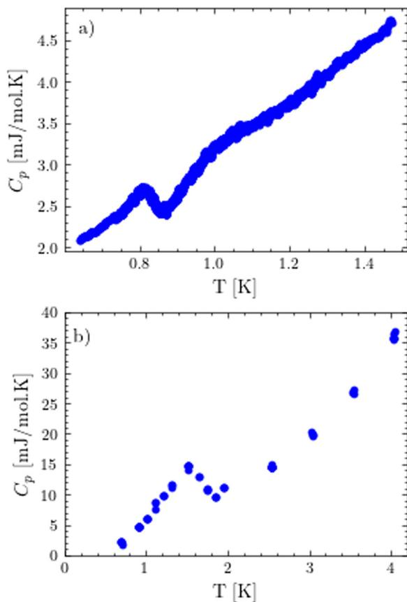
Fig. 5 The superconducting anomaly in the (a) HCP and (b) BCC materials. Since the transition temperature of the HCP system is near the reliable limit of the  $^3\text{He}$  apparatus, Quantum Design's dual slope analysis routine was used, which gives more data points.
