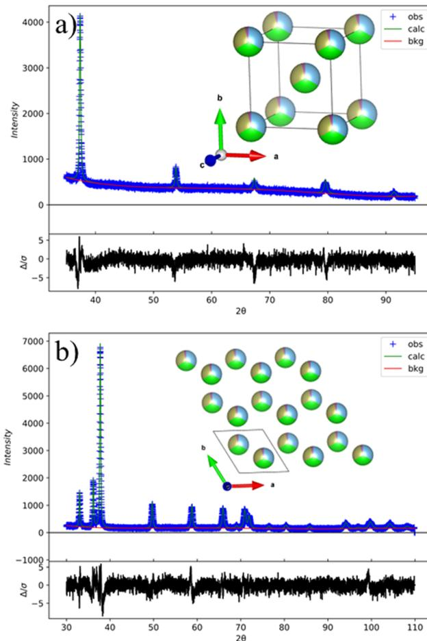
Fig. 1 Bulk polycrystalline X-ray diffraction patterns for the (a) BCC and (b) HCP phases. (Cu  $K\alpha$  radiation) Their relative structures are presented as well showing 31.7% Ti, 31.7% Zr, 31.7% Hf, and 5% Sc.
