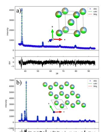
Fig. 1 Bulk polycrystalline X-ray diffraction patterns for the (a) BCC and (b) HCP phases. (Cu Kα radiation) Their relative structures are presented as well showing 31.7% Ti, 31.7% Zr, 31.7% Hf, and 5% Sc.
