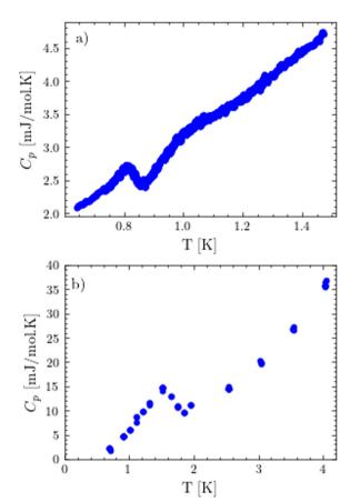
Fig. 5 The superconducting anomaly in the (a) HCP and (b) BCC materials. Since the transition temperature of the HCP system is near the reliable limit of the <sup>3</sup>He apparatus, Quantum Design's dual slope analysis routine was used, which gives more data points.
