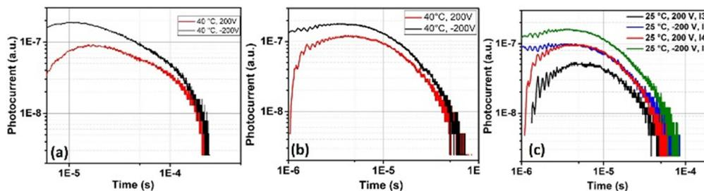
Fig. 6 Ambipolar transient photocurrent curves for (a) **9**, (b) **11** and (c) **11** with two different laser intensities, *i.e.*  $I_3 \approx 3\%$  (equivalent to 3 mW) and  $I_4 \approx 4\%$  (equivalent to 4 mW).
