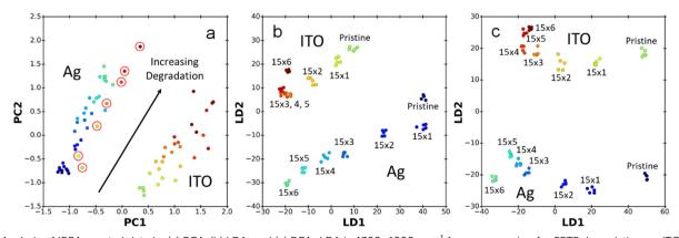
Fig. 6 Analysis of IRRA spectral data by (a) PCA, (b) LDA, and (c) PCA-LDA in 1300-1900 cm<sup>-1</sup> frequency region for FBTF degradation on ITO and Aq under sequential 15 min exposures to a 75 W Xe lamp. Samples color-coded by substrate type and exposure time. Red circles in PCA results indicate outlier data set for FBTF on one ITO sample; this set retained for subsequent LDA and PCA-LDA analyses.
