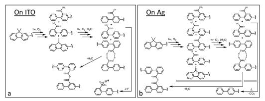
Fig. 2 Proposed pathways for oxidative degradation of 9,9-dimethylfluorene subunit of FBTF on (a) ITO and (b) Ag based on IRRAS results
