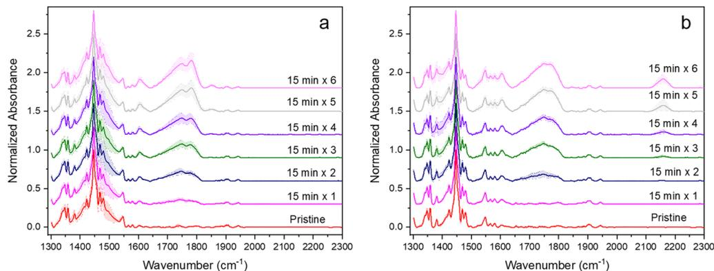
Fig. 5 Normalized IRRA spectra of pristine FBTF thin films and those exposed to a series of six 15-min exposures on (a) ITO and (b) Ag. Spectra collected with 2000 scans at  $4\text{ cm}^{-1}$  resolution. Intensities plotted as normalized values with respect to the  $1446\text{ cm}^{-1}$  band; stacked spectra plotted with offset of 0.3 normalized a.u. Shaded regions represent the variance in normalized spectral intensities across the sample set for each substrate.
