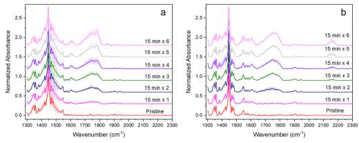
Fig. 5 Normalized IRRA spectra of pristine FBTF thin films and those exposed to a series of six 15-min exposures on (a) ITO and (b) Ag. Spectra collected with 2000 scans at 4 cm<sup>-1</sup> resolution. Intensities plotted as normalized values with respect to the 1446 cm<sup>-1</sup> band; stacked spectra plotted with offset of 0.3 normalized a.u. Shaded regions represent the variance in normalized spectral intensities across the sample set for each substrate.
