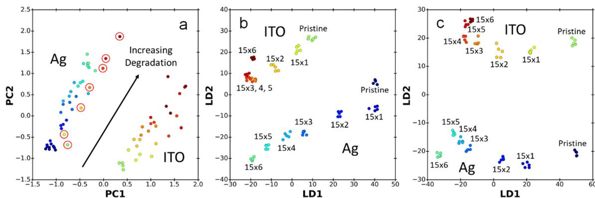
Fig. 6 Analysis of IRRA spectral data by (a) PCA, (b) LDA, and (c) PCA-LDA in  $1300\text{--}1900\text{ cm}^{-1}$  frequency region for FBTF degradation on ITO and Ag under sequential 15 min exposures to a 75 W Xe lamp. Samples color-coded by substrate type and exposure time. Red circles in PCA results indicate outlier data set for FBTF on one ITO sample; this set retained for subsequent LDA and PCA-LDA analyses.
