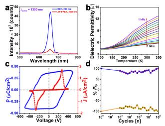
Fig. 2 (a) SHG profile of AP·FPBA compared to standard KDP sample. (b) Dielectric permittivity vs. temperature profile of AP·FPBA. (c) P-E hysteresis loop for AP-FPBA. (d) The ferroelectric fatigue test of AP-FPBA up to 10<sup>6</sup> cycles.
