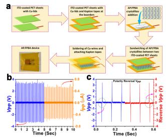
Fig. 4 (a) Schematic for the preparation of AP-FPBA device for piezoelectric measurements. (b) Open circuit peak-to-peak voltage and short-circuit current of AP·FPBA. (c) The switching of the  $V_{PP}$  profile of AP·FPBA device upon polarity reversal. The shifted time axis provided is a guide to the eye.
