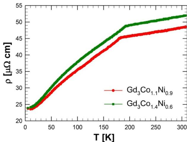
Fig. 7 Zero-field electrical resistivity for the  $\text{Gd}_3\text{Co}_{1.1}\text{Ni}_{0.9}$  and  $\text{Gd}_3\text{Co}_{1.4}\text{Ni}_{0.6}$  compounds as a function of temperature in the range of 5–300 K.
