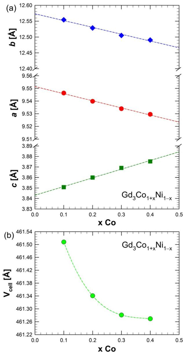
Fig. 5 Trend of the lattice parameters ( $a$ ,  $b$ ,  $c$ ) (a) and unit cell volume ( $V_{cell}$ ) (b) as a function of the Co content  $x$  in the orthorhombic  $Y_3Co_2$ -type  $Gd_3Co_{1+x}Ni_{1-x}$  ( $x = 0.1, 0.2, 0.3, 0.4$ ) series.
