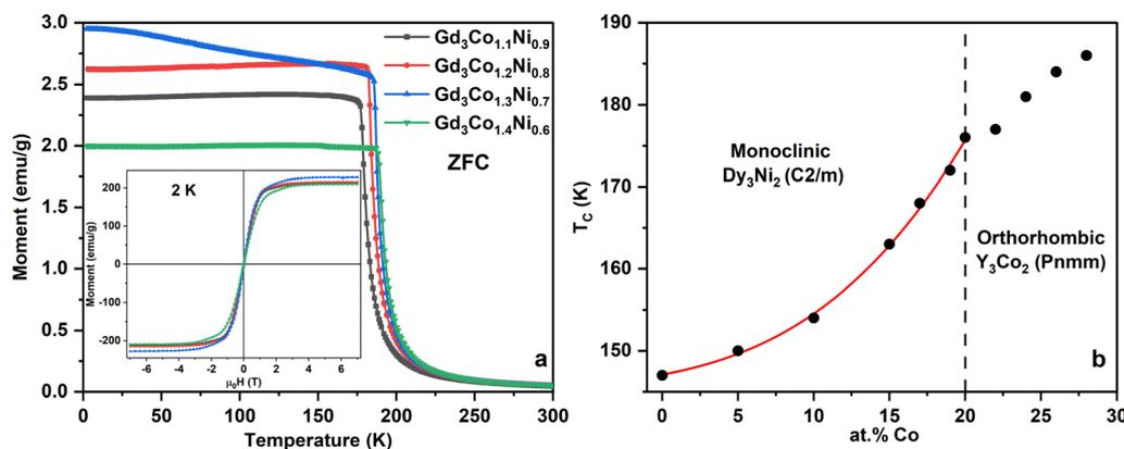
Fig. 8 ZFC magnetization at  $\mu_0 H = 0.01$  T for the four  $\text{Gd}_3\text{Co}_{1+x}\text{Ni}_{1-x}$  ( $x = 0.1, 0.2, 0.3, 0.4$ ) compounds (a); the inset shows the isothermal magnetization,  $M(H)$ , at  $T = 2$  K. Variation of Curie temperature ( $T_C$ ) as a function of the Co content (in at%) for both monoclinic  $\text{Dy}_3\text{Ni}_2$ -type  $\text{Gd}_3\text{Co}_y\text{Ni}_{2-y}$  and orthorhombic  $\text{Y}_3\text{Co}_2$ -type  $\text{Gd}_3\text{Co}_{1+x}\text{Ni}_{1-x}$  (b).
