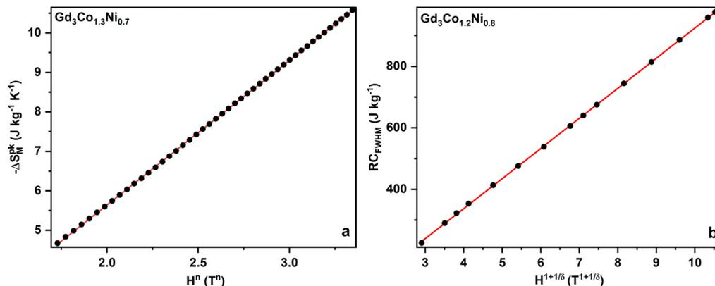
Fig. 11 Field dependence of the magnetic entropy change peak for  $\text{Gd}_3\text{Co}_{1.3}\text{Ni}_{0.7}$  (a) and  $\text{RC}_{\text{FWHM}}$  for  $\text{Gd}_3\text{Co}_{1.2}\text{Ni}_{0.8}$  (b); the red line is a linear fit to be used as a visual guide.
