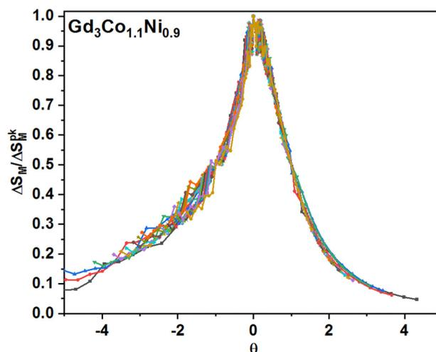
Fig. 13 Universal curve for the  $\text{Gd}_3\text{Co}_{1.1}\text{Ni}_{0.9}$  compound.
