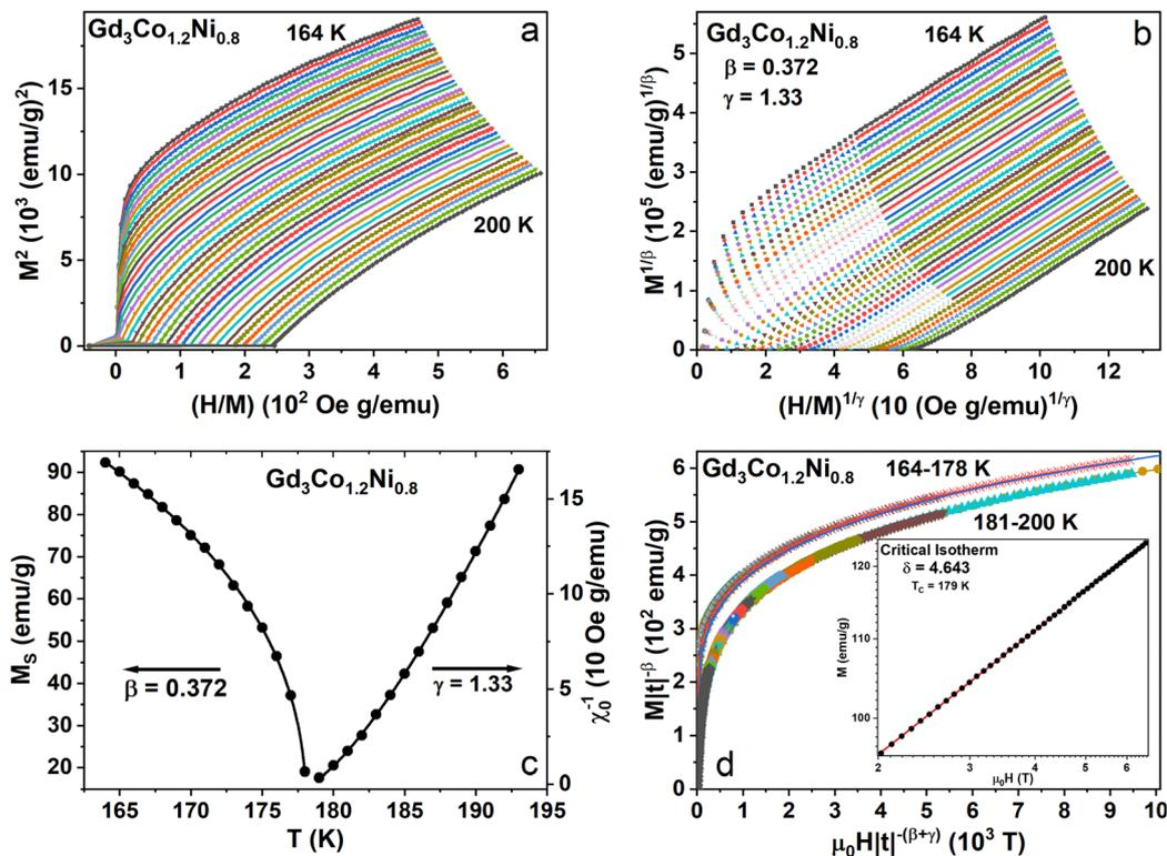
Fig. 9 Critical behavior analysis for  $\text{Gd}_3\text{Co}_{1.2}\text{Ni}_{0.8}$ . Arrott plot representation (a); modified Arrott plot representation using the correct critical exponents (b); fitting of  $M_S$  and  $\chi_0^{-1}$  to eqn (1) and (2) respectively (c); magnetic equation of state, with the inset showing the fitting of the critical isotherm to eqn (3) (d).
