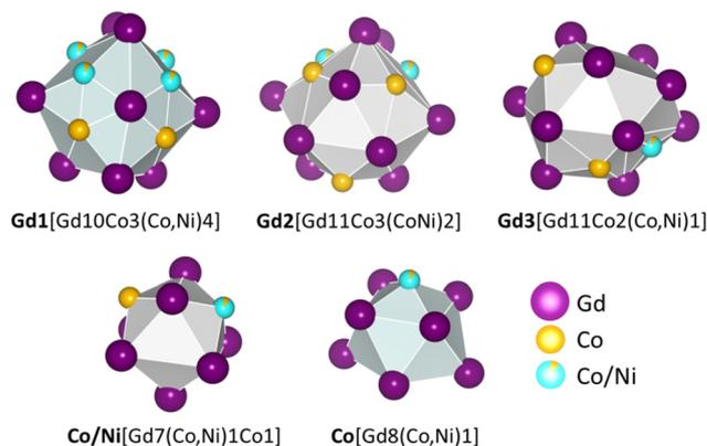
Fig. 4 Coordination polyhedra around Gd1, Gd2, Gd3, Co/Ni and Co atoms corresponding to the first coordination sphere for  $d_{\text{obs}}/\sum r_{\text{M}} \leq 1.166$  in  $\text{Gd}_3\text{Co}_{1.1}\text{Ni}_{0.9}$ .
