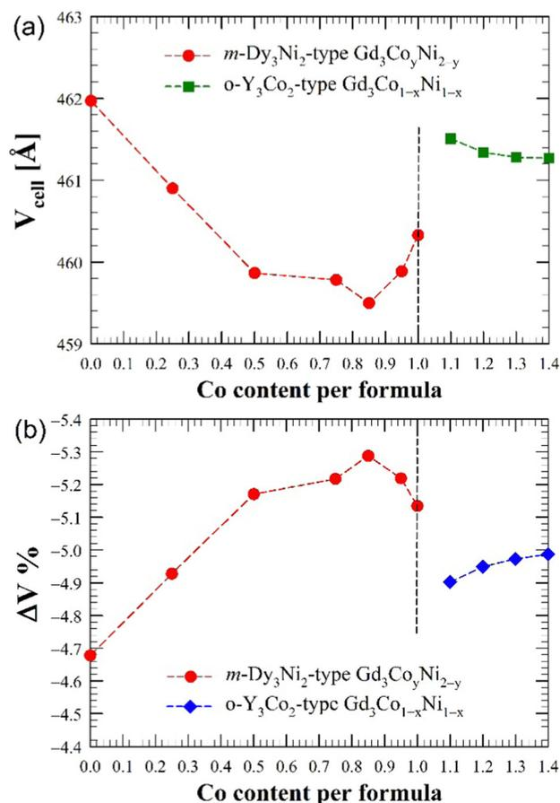
Fig. 6 Unit cell volume ( $V_{cell}$ ) (a) and formation volume ( $\Delta V$ ) (b) as a function of the Co content  $y$  in the monoclinic  $Dy_3Ni_2$ -type  $Gd_3Co_yNi_{2-y}$  ( $y = 0, 0.25, 0.50, 0.75, 0.85, 0.95, 1.00$ ) and in the orthorhombic  $Y_3Co_2$ -type  $Gd_3Co_{1+x}Ni_{1-x}$  ( $x = 0.1, 0.2, 0.3, 0.4$ ) compounds.
