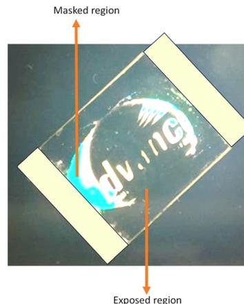
Fig. 19 Optical storage device fabricated using **CB11AZ**, where dimers were used as the guest molecule and the liquid crystal E7 was used as the host molecule. One can see from the device that the exposed region corresponds to the UV illumination (dark state) and the masked region is corresponding to that UV-protected area through the mask (dark state).
