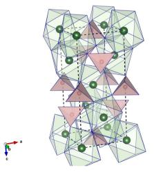
Fig. 2 The crystal structure model of the tetragonal unit cell of LuPO<sub>4</sub> in polyhedral presentation: green atoms - Lu, red atoms - P; oxygen atoms are located at the vertices of polyhedra, but not presented for the sake of the image clarity. The figure has been prepared using VESTA software.
