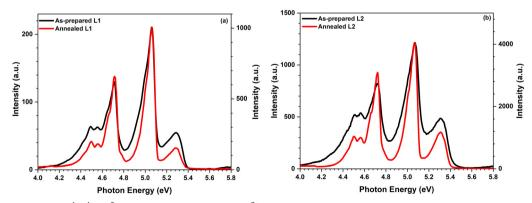
Fig. 8 Effect of annealing on  $4f^15d^1 \rightarrow 4f^2$  luminescence intensities of  $Pr^{3+}$  ions under intra-center excitation at 6.54 eV of the as-prepared and annealed LuPO<sub>4</sub>:Pr<sup>3+</sup> (1%) nanocrystals at 6.8 K. The intensities of the as-prepared and annealed L1, L2 samples are shown on the left and right intensity axes, respectively.
