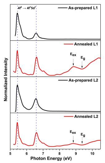
Fig. 7 TI PL excitation spectra of the as-prepared and annealed LuPO<sub>4</sub>:Pr<sup>3+</sup> (1%) nanocrystals at 6.8 K recorded for the  $4f^15d^1 \rightarrow {}^3H_5$ luminescence peaked at 5.06 eV (the signal is integrated for the emission energy range from 4.9 to 5.1 eV).
