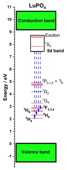
Fig. 5 Schematic representation of the fundamental electronic structure of LuPO<sub>4</sub>:Pr<sup>3+</sup>, based on P. Dorenbos' methodology. <sup>17,41</sup> The host nearedge energy bands, impurity levels and the  $Pr^{3+} 4f^15d^1 \rightarrow 4f^2$  transitions (blue arrows) are illustrated.
