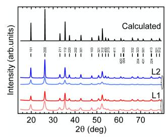
Fig. 1 XRD patterns of as-prepared (lower curve) and annealed (upper curve) LuPO<sub>4</sub>:Pr<sup>3+</sup> (1%) powder synthesized in L1 (30% DMSO-70% water) solvent and L2 (50% DMSO-50% water) solvent. The calculated diffraction pattern including the indices of reflections of tetragonal LuPO<sub>4</sub> is shown at the topmost part of the figure.
