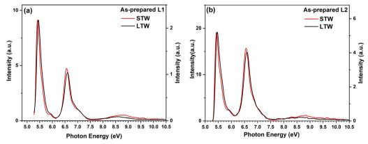
Fig. 11 Time resolved PL excitation spectra of the as-prepared LuPO<sub>4</sub>:  $Pr^{3+}$  (1%) L1 (a) and L2 (b) nanocrystals recorded at 6.8 K for the  $4f^{1}5d^{1} \rightarrow {}^{3}H_{5}$ luminescence at 5.06 eV in the STW ( $\delta t = 0$  and  $\Delta t = 4$  ns) and LTW ( $\delta t = 4$  and  $\Delta t = 20$  ns). The spectra are normalized to the highest intensity of the excitation band for better comparison
