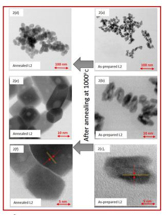
Fig. 4 The first row [1(a), 1(d), 2(d) and 2(a)] STEM images are of different LuPO<sub>4</sub>:Pr<sup>3+</sup> (1%) nanocrystal families displaying uniformity of the particles. The middle row images [1(b), 1(e), 2(b) and 2(e)] are high resolution TEM images for smaller  $LuPO_4$ :  $Pr^{3+}$  (1%) nanocrystal agglomerates. The bottom row [1(c), 1(f), 2(c) and 2(f)] shows high-resolution STEM images taken at a 5 nm resolution, with visible lattice fringes indicating crystallinity.
