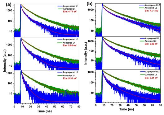
Fig. 10 Effect of annealing on the  $4f^15d^1 \rightarrow {}^3H_{4^+}{}^3H_{5^+}{}^3H_6$  luminescence decay of the  $Pr^{3^+}$  ions for (a) L1 and (b) L2 nanocrystals, recorded under the intracenter excitation of the Pr3+ ion by the 6.54 eV photons at 7 K. Experimental data (green and blue lines) are fitted by the bi-exponential decay function, which is shown by red lines. The decay curves are normalized at their maxima for better comparison.
