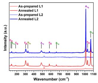
Fig. 3 Raman spectra of the as-prepared and annealed LuPO<sub>4</sub>:Pr<sup>3+</sup> nanocrystals recorded at 300 K. The band at 520 cm<sup>-1</sup> in the spectra of as-prepared samples is related to the silicon substrate.
