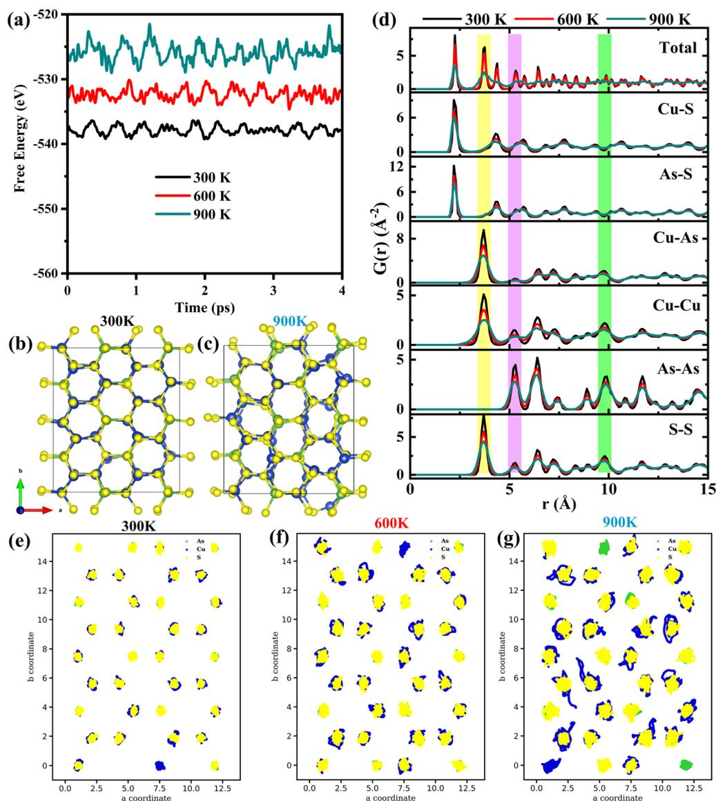
**Fig. 2** (a) Evolution of free energy at different simulation temperatures. The final structures at (b) 300 K and (c) 900 K. (d) Averaged total and partial pair distribution functions. The atomic trajectory of atoms at (e) 300 K, (f) 600 K and (g) 900 K, respectively.
