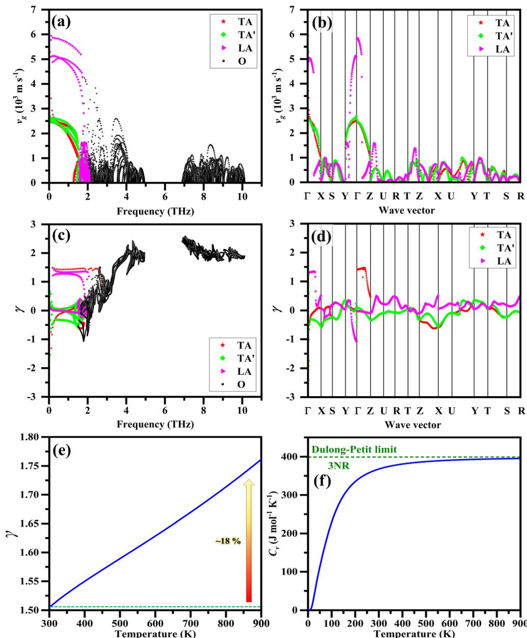
Fig. 4 Group velocity as a function of (a) frequency and (b)  $q$ -points. The Grüneisen parameter as a function of (c) frequency, (d)  $q$ -points and (e) temperature. (f) Specific heat against temperature.
