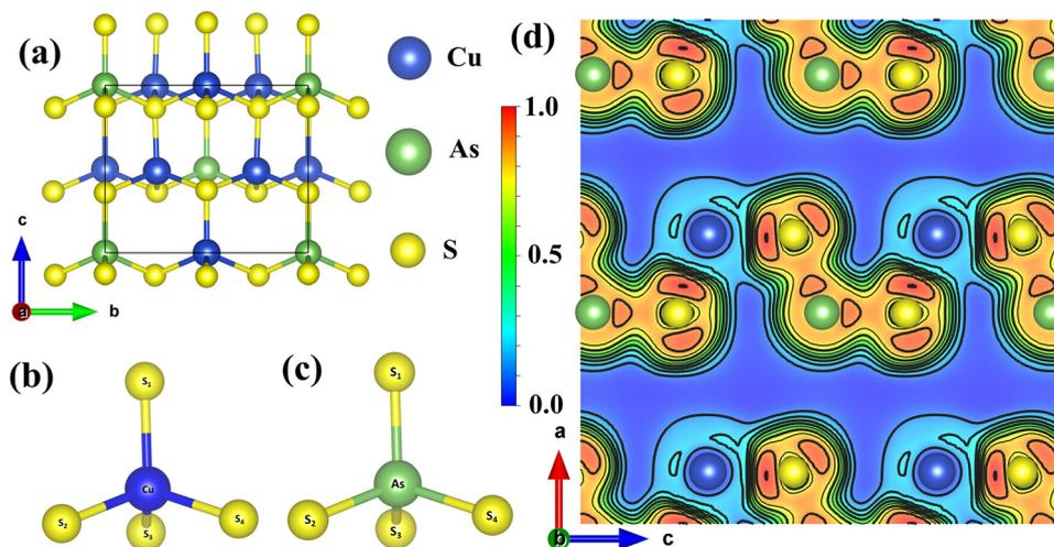
Fig. 1 (a) Crystal structure along the  $a$ -axis, tetrahedral coordination of (b) Cu–S and (c) As–S and (d) 2D electron localization function for the  $2 \times 2 \times 2$  supercell projected along the (0 1 0) plane.
