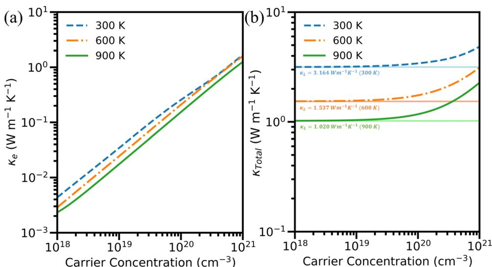
Fig. 9 (a) Electronic and (b) total thermal conductivity of hole-doped  $\text{Cu}_3\text{AsS}_4$  at different temperatures. The light-colored lines indicate the corresponding lattice thermal conductivity at specific temperatures obtained *via* the PBTE-Iterative approach.
