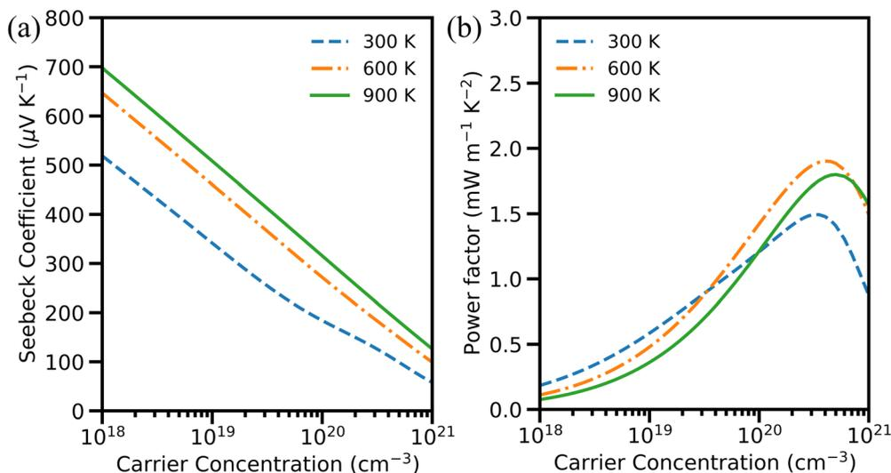
Fig. 8 (a) Seebeck coefficient and (b) power factor of hole-doped  $\text{Cu}_3\text{AsS}_4$  against carrier concentration at different temperatures.
