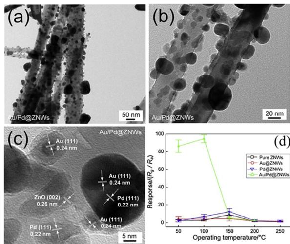
Fig. 9 (a) and (b) TEM and (c) HRTEM images of AuPd–ZnO NWs and (d) response of gas sensors to 1 ppm NO<sub>2</sub> versus temperature. Reproduced with permission from Elsevier, ref. 60.
