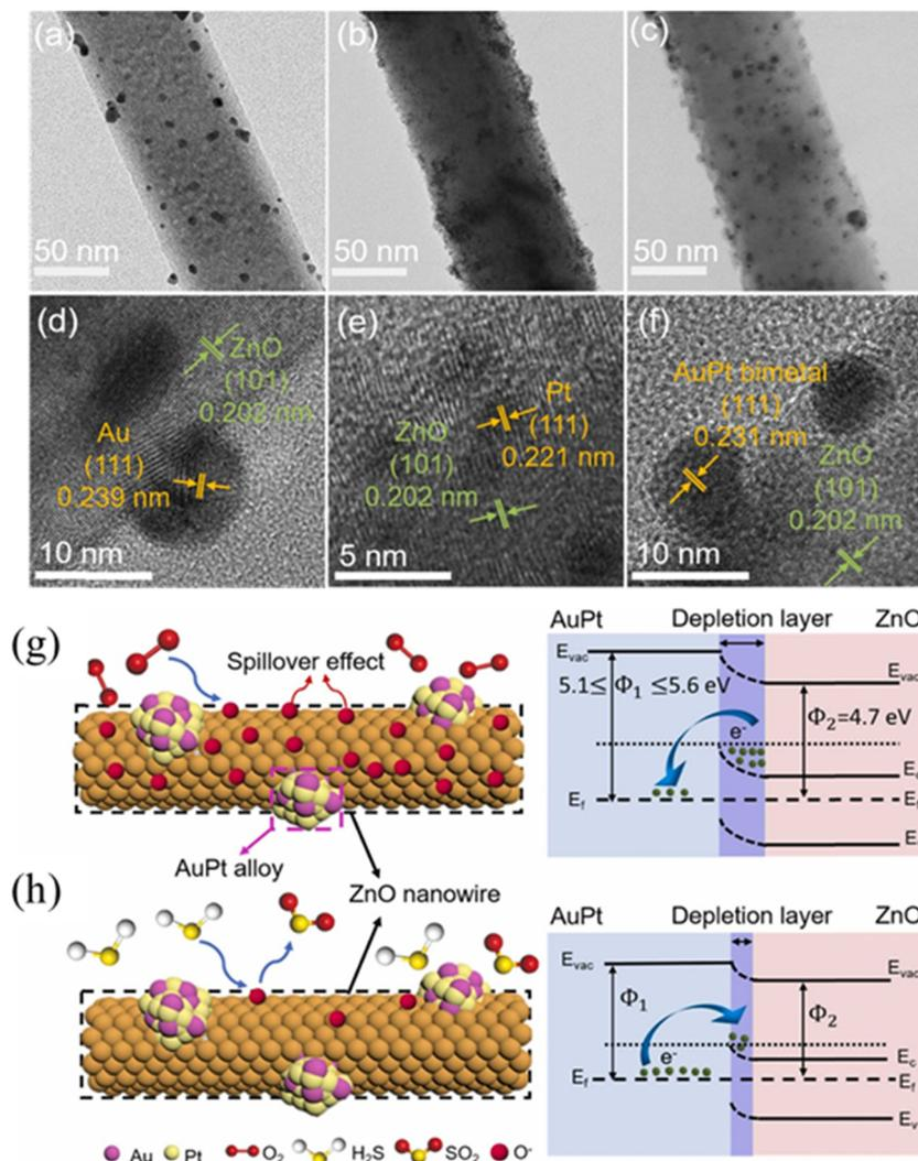
Fig. 16 TEM and HRTEM images of (a) and (d) Au-, (b) and (e) Pt-, and (c) and (f) PtAu-decorated ZnO NWs. The underlying  $\text{H}_2\text{S}$  sensing mechanism of the PtAu-decorated ZnO NWs in (g) air and (h)  $\text{H}_2\text{S}$  gas. Reproduced with permission from Elsevier, ref. 76.
