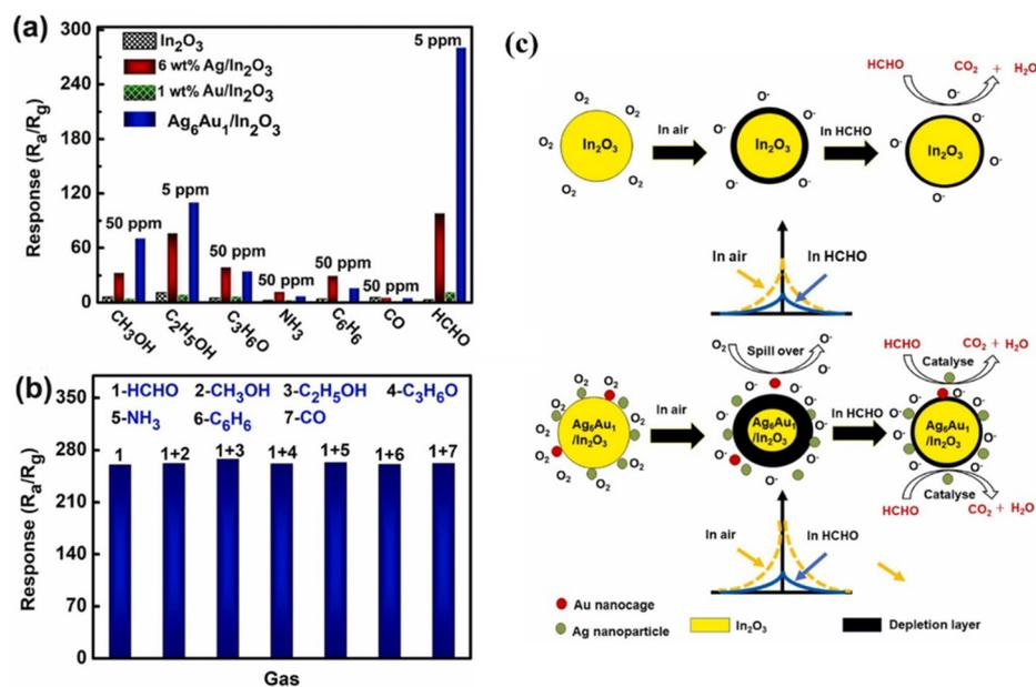
Fig. 23 (a) Selectivity of various gas sensors at 170 °C; (b) discrimination test of the Ag<sub>6</sub>Au<sub>1</sub>/In<sub>2</sub>O<sub>3</sub> sensor to the response of mixed gas with 5 ppm HCHO and 5 ppm other interference gases; (c) HCHO sensing mechanism on the surfaces of In<sub>2</sub>O<sub>3</sub> and Ag<sub>6</sub>Au<sub>1</sub>/In<sub>2</sub>O<sub>3</sub> sensors. Reproduced with permission from Elsevier, ref. 98.
