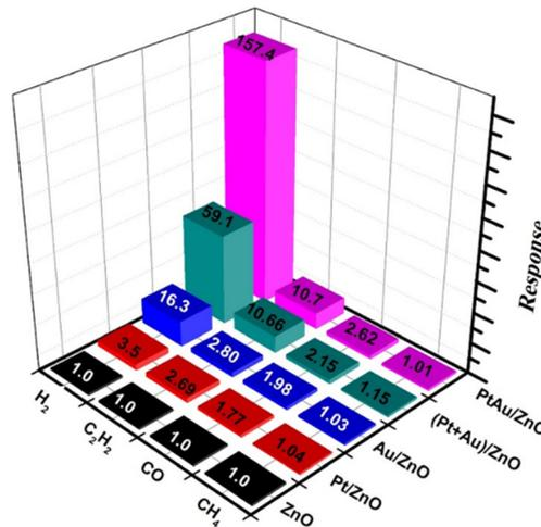
Fig. 15 Selectivity of various gas sensors to 250 ppm gases at  $130^\circ\text{C}$ . Reproduced with permission from Elsevier, ref. 75.
