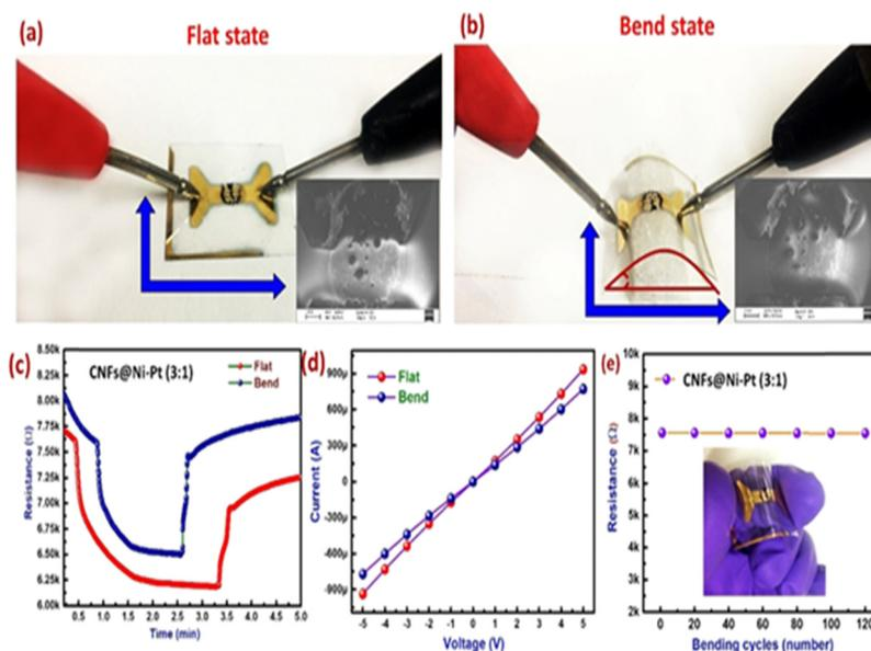
Fig. 17 CNFs@Ni–Pt sensor (3 : 1): (a) flat state and (b) bent state; (c) sensing performance to 1% H<sub>2</sub> at flat and bent states, (d) current–voltage characteristics, and (e) resistance of the flexible CNF@Ni–Pt (3 : 1) sensor versus the number of bending cycles. Reproduced with permission from American Chemical Society, ref. 82.
