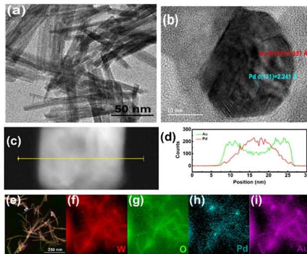
Fig. 12 (a) TEM image of  $\text{W}_{18}\text{O}_{49}$  NWs, (b) HRTEM image of  $\text{W}_{18}\text{O}_{49}$  NWs/BNPs-2 and (c) and (d) EDS elemental line and (e)–(i) surface scans of  $\text{W}_{18}\text{O}_{49}$  NWs/BNPs-2. Reproduced with permission from Elsevier, ref. 72.
