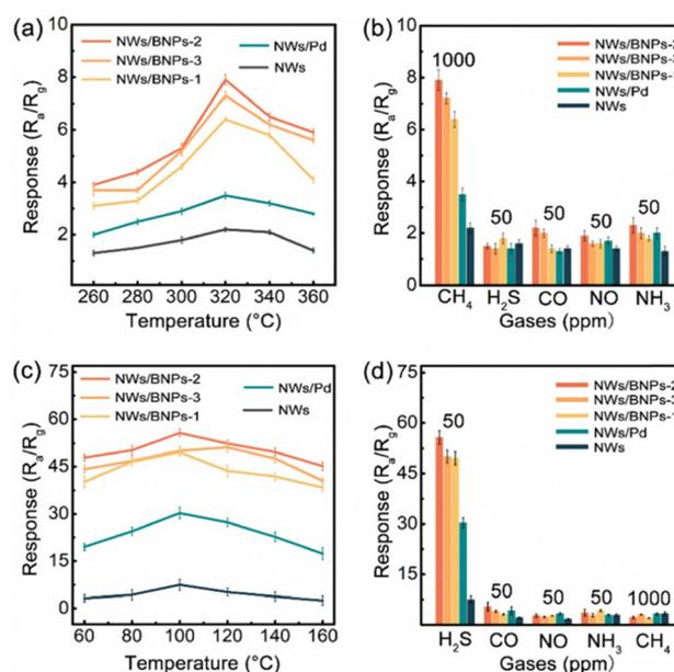
Fig. 13 Response of different sensors to (a) 1000 ppm  $\text{CH}_4$  and (c) 50 ppm  $\text{H}_2\text{S}$  versus temperature; selectivity of  $\text{W}_{18}\text{O}_{49}$  NWs/BNPs-2 at (b) 320 °C and (d) 100 °C. Reproduced with permission from Elsevier, ref. 72.
