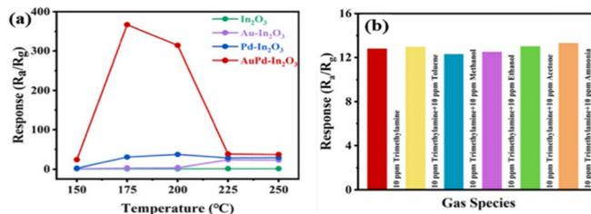
Fig. 10 (a) Gas sensing response of various gas sensors to 100 ppm C<sub>3</sub>H<sub>9</sub>N; (b) selectivity of the AuPd–In<sub>2</sub>O<sub>3</sub> sensor to 10 ppm gas and 10 ppm C<sub>3</sub>H<sub>9</sub>N. Reproduced with permission from Elsevier, ref. 61.
