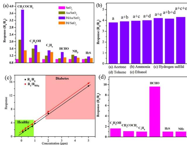
Fig. 11 Sensing tests of the AuPd/ $\text{SnO}_2$  sensor: (a) selectivity graph; (b) discrimination test of the response to the mixed gas (1 ppm  $\text{C}_3\text{H}_6\text{O}$  and 1 ppm other interference gases); (c) response to different concentrations of  $\text{C}_3\text{H}_6\text{O}$  in a 94% RH environment at 250  $^\circ\text{C}$ ; and (d) AuPd/ $\text{SnO}_2$  sensor selectivity at 110  $^\circ\text{C}$ . Reproduced with permission from Elsevier, ref. 65.
