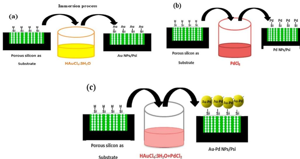
Fig. 7 Synthesis of (a) Au-, (b) Pd-, and (c) AuPd-decorated P-Si. Reproduced with permission from Elsevier, ref. 50.
