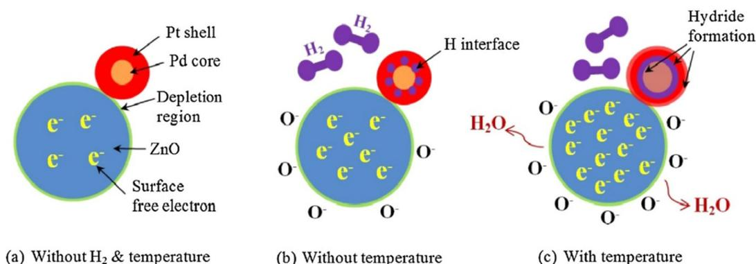
Fig. 18  $\text{H}_2$  sensing mechanism of ZnO NRs decorated with Pt/Pd bimetallic core–shell quantum dots (QDs): (a) in the absence of  $\text{H}_2$  at low temperature, (b) in the presence of  $\text{H}_2$  at low temperature, and (c) in the presence of both  $\text{H}_2$  and elevated temperature. Reproduced with permission from American Chemical Society, ref. 86.
