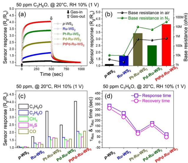
**Fig. 20** (a) Sensing plots of various gas sensors to C<sub>3</sub>H<sub>6</sub>O, (b) corresponding response, and baseline resistance in air and N<sub>2</sub>; (c) selectivity curves, and (d) response and recovery times. Reproduced with permission from Elsevier, ref. 92.
