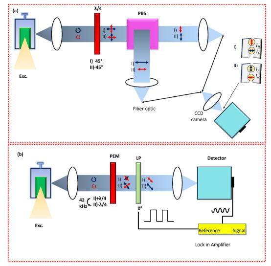
Fig. 7 (a) and (b) Different types of instrument setup for CPL detection. Exc. is excitation, LP is a linear polarizer, PBS is a polarizing beam splitter, I1 is the intensity of LCP,  $I_R$  is the intensity of RCP, and PEM is photoelastic modulator. The blue curve arrow is LCP, and the red curve is RCP. Explanation for the diagrams is in the main text. (redrawn from ref. 108)
