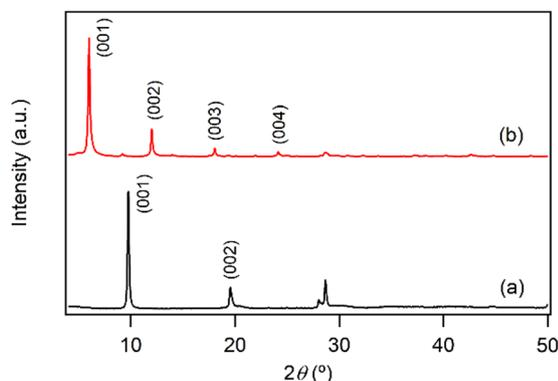
Fig. 1 Powder XRD patterns of (a) LYH:Eu and (b) NA-LYH:Eu.
