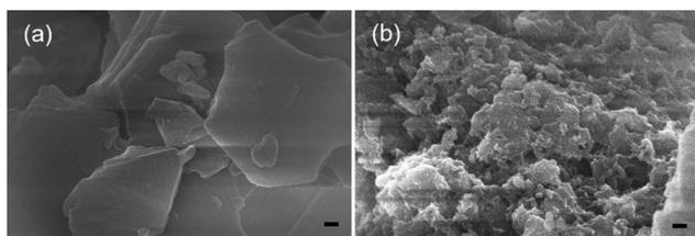
Fig. 8 FE-SEM images of NA-LYH:Eu particles (a) before and (b) after release reaction in PBS for 24 h (bar = 100 nm).
