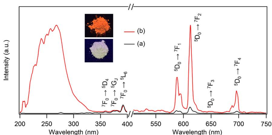
Fig. 3 Excitation and emission spectra of (a) LYH:Eu ( $\lambda_{\text{em}} = 613 \text{ nm}$ ,  $\lambda_{\text{ex}} = 392 \text{ nm}$ ) and (b) NA-LYH:Eu ( $\lambda_{\text{em}} = 613 \text{ nm}$ ,  $\lambda_{\text{ex}} = 268 \text{ nm}$ ). Inset: Photographs of LYH:Eu and NA-LYH:Eu under a  $254 \text{ nm}$  UV lamp.
