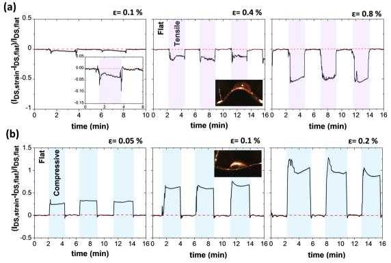
Fig. 3 Real-time  $I_{DS}$  current monitoring (baseline corrected) of a diF-TES-ADT:PS EGOFET employing Milli-Q water as electrolyte and fixing  $V_{DS}$  = -0.2 V and  $V_{GS} = -0.2$  V, applying (a) cyclic tensile strain (purple regions) equal to 0.1, 0.4 and 0.8%, and (b) cyclic compressive strain (blue regions) equal to 0.05, 0.1 and 0.2%
