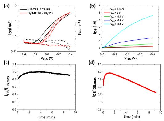
Fig. 2 (a) Transfer characteristics ( $V_{DS} = -0.1 \text{ V}$ ) and their corresponding source-gate current (dashed lines) for diF-TES-ADT:PS (black curves) and  $C_8O$ -BTBT-OC<sub>8</sub> (red curves) EGOFETs. (b) Output characteristics ( $V_{GS} = 0.05, 0, -0.1, -0.2, -0.4$  V) of diF-TES-ADT:PS EGOFETs. Real-time  $I_{DS}$  monitoring of a diF-TES-ADT:PS EGOFET (c) and  $C_8O$ -BTBT-O $C_8$ :PS EGOFET (d) fixing  $V_{DS} = V_{GS} = -0.2$  V.
