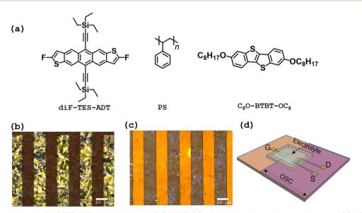
Fig. 1 (a) Molecular structure of diF-TES-ADT, polystyrene, and C<sub>8</sub>O-BTBT-OC<sub>8</sub>. Polarized optical microscopy images of (b) diF-TES-ADT:PS, and (c) C<sub>8</sub>O-BTBT-OC<sub>8</sub>:PS thin films coated on Kapton substrates. The scale bar of POM images is 50 µm. (d) Schematic representation of the EGOFET device configuration employed.
