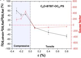
Fig. 4 Changes in current (black line) and gauge factor (red line) while applying compressive and tensile strain for (a) diF-TES-ADT:PS and (b) C<sub>8</sub>O-BTBT-OC<sub>8</sub>:PS EGOFET employing Milli-Q water as electrolyte in real-time current monitoring. The error bars correspond to the average and standard deviation of at least three different cycles for each applied strain value
