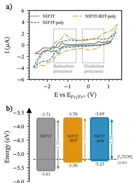
**Fig. 2** (a) Cyclic voltammogram comparison between **NIP3T-poly** and **NIP3T-BDT-poly** organic conjugated polymers. (b) Molecular orbitals energy levels diagram of the studied  $\pi$ -conjugated polymers and the corresponding **NIP3T** molecular analogue in this work.
