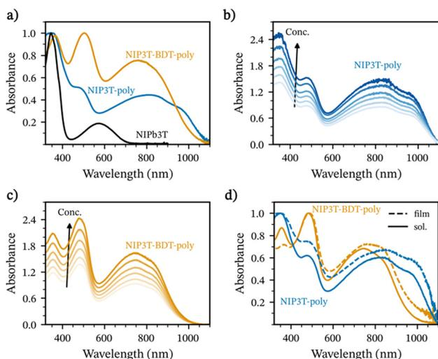
**Fig. 1** (a) Normalized UV-vis-NIR spectra of chlorobenzene fractions of **NIP3T**, **NIP3T-poly** and **NIP3T-BDT-poly** in chlorobenzene, (b) and (c) concentration-dependent experiments for both polymers **NIP3T-poly** and **NIP3T-BDT-poly** respectively and (d) Normalized thin-film absorption spectra of these new oligothiophene-naphthalimide polymers. For (c) and (b), concentrations increase from 0.17 mg mL<sup>-1</sup> to 0.30 mg mL<sup>-1</sup>.
