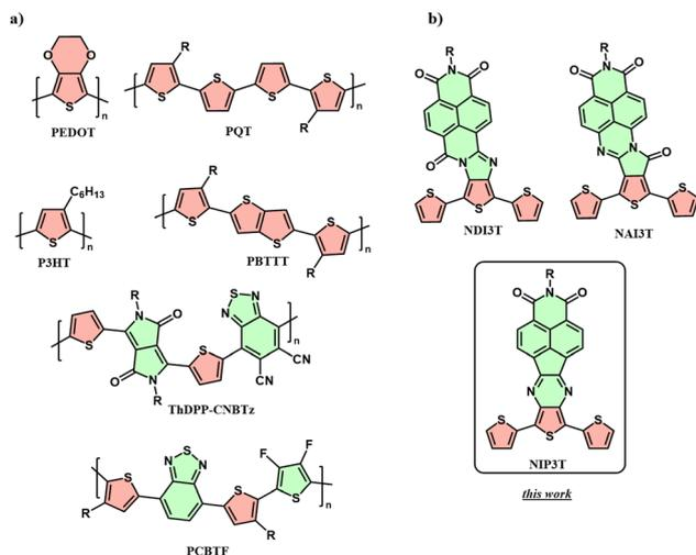
**Chart 1** Chemical structures of (a) conventional conjugated polymers used in the field of thermoelectrics and (b) building blocks for polymers studied in this work.
