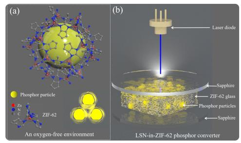
Fig. 7 (a) Mechanism of the organic-inorganic glass ZIF-62 providing an oxygen-free sintering environment for protecting LSN:Ce phosphors. (b) Schematic of the laser-driven sandwich-structured LSN-in-ZIF-62 phosphor converter.
