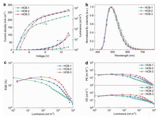
Fig. 5 (a) Current density and luminance versus voltage (J-V-L) characteristics. (b) EL spectra at a luminance of 1000 cd m<sup>-2</sup>. (c) EQE as a function of luminance. (d) PE and CE as a function of luminance.
