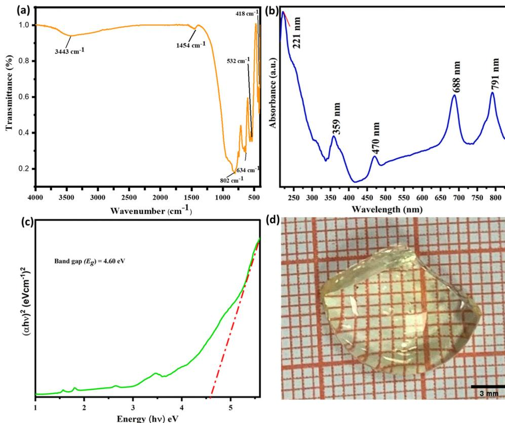
Fig. 3 (a) FTIR spectra of  $\text{CaAl}_4\text{O}_7:\text{Tm}^{3+}$  phosphor material. (b) Absorption spectra and (c) Tauc plot of  $\text{Ca}_{(1-x)}\text{Al}_4\text{O}_7:x\text{Tm}^{3+}$  ( $x = 0.03$ ) phosphor material (d) Fabricated phosphor-in-glass based on optimized  $\text{CaAl}_4\text{O}_7:\text{Tm}^{3+}$  phosphor.
